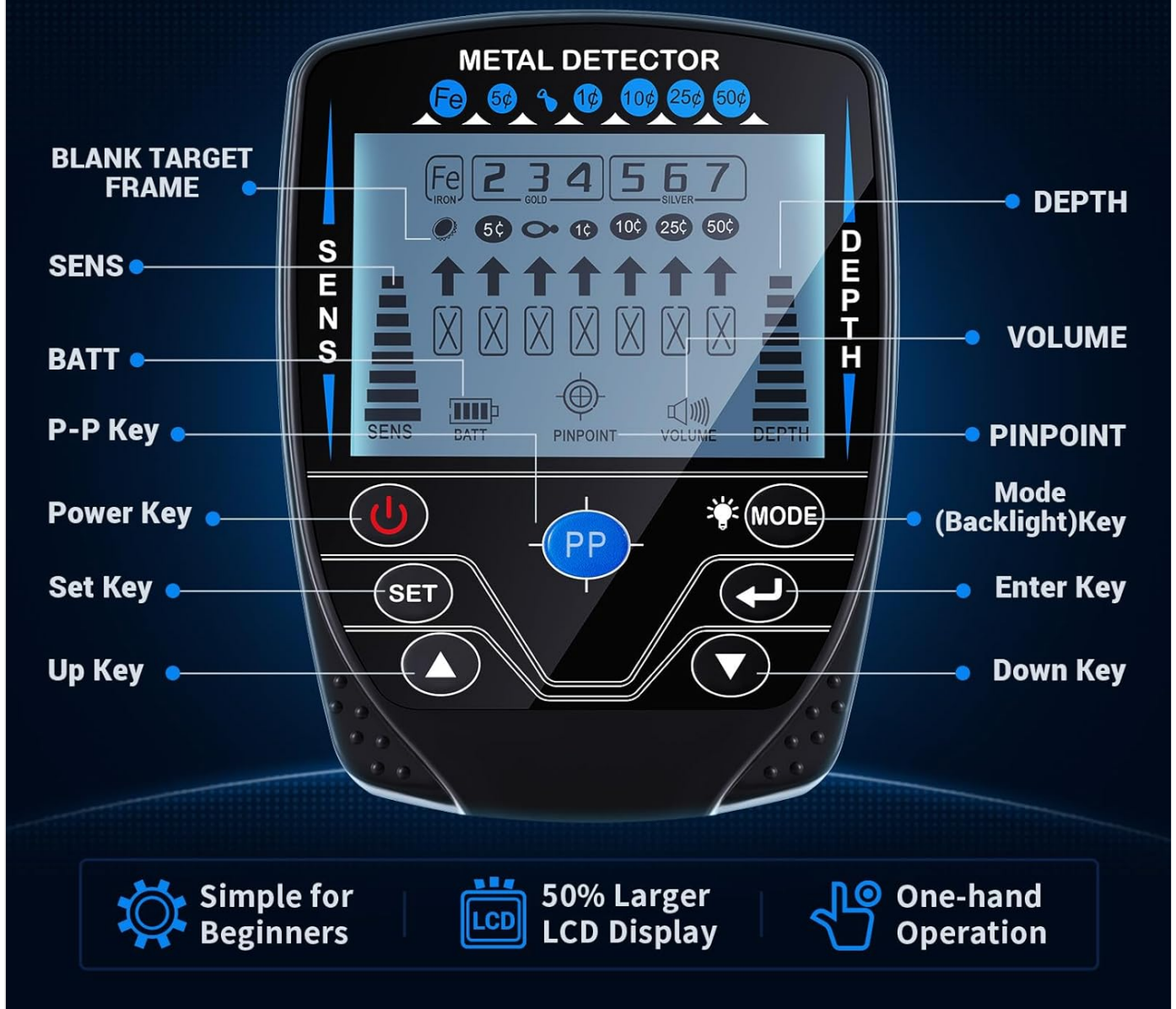
Figure 3.1: The intuitive LCD screen displays target information, depth, sensitivity, and battery status. Key buttons include Power, Set, Up, Down, Mode (for backlight), Pinpoint (PP), and Enter.
