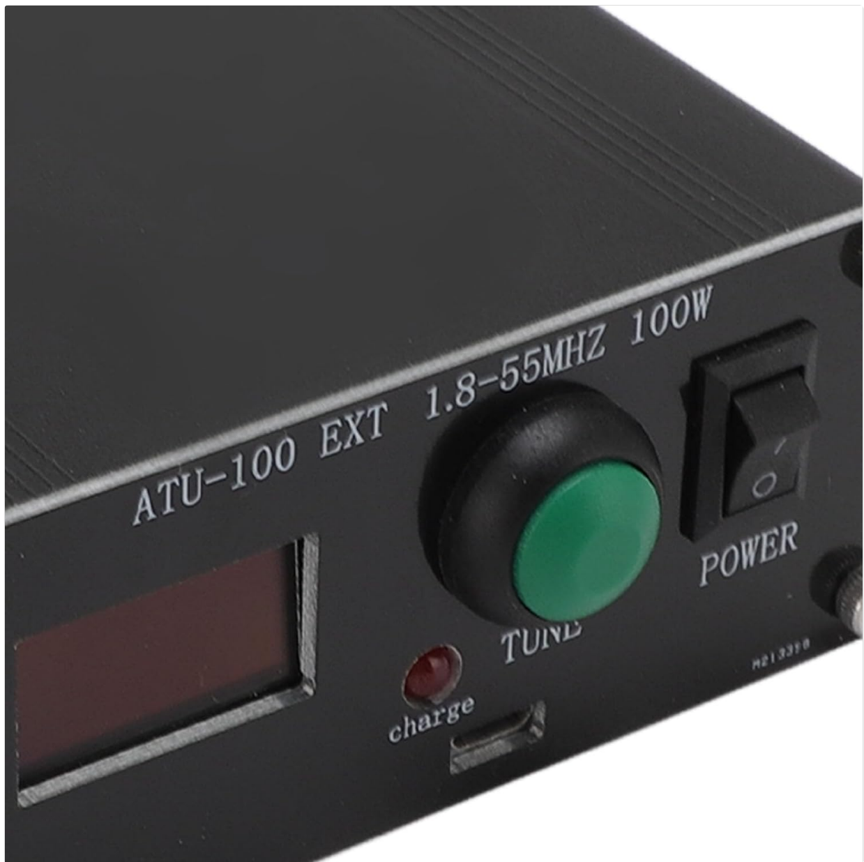
Figure 3: Detailed view of the control panel with display and TUNE button.
