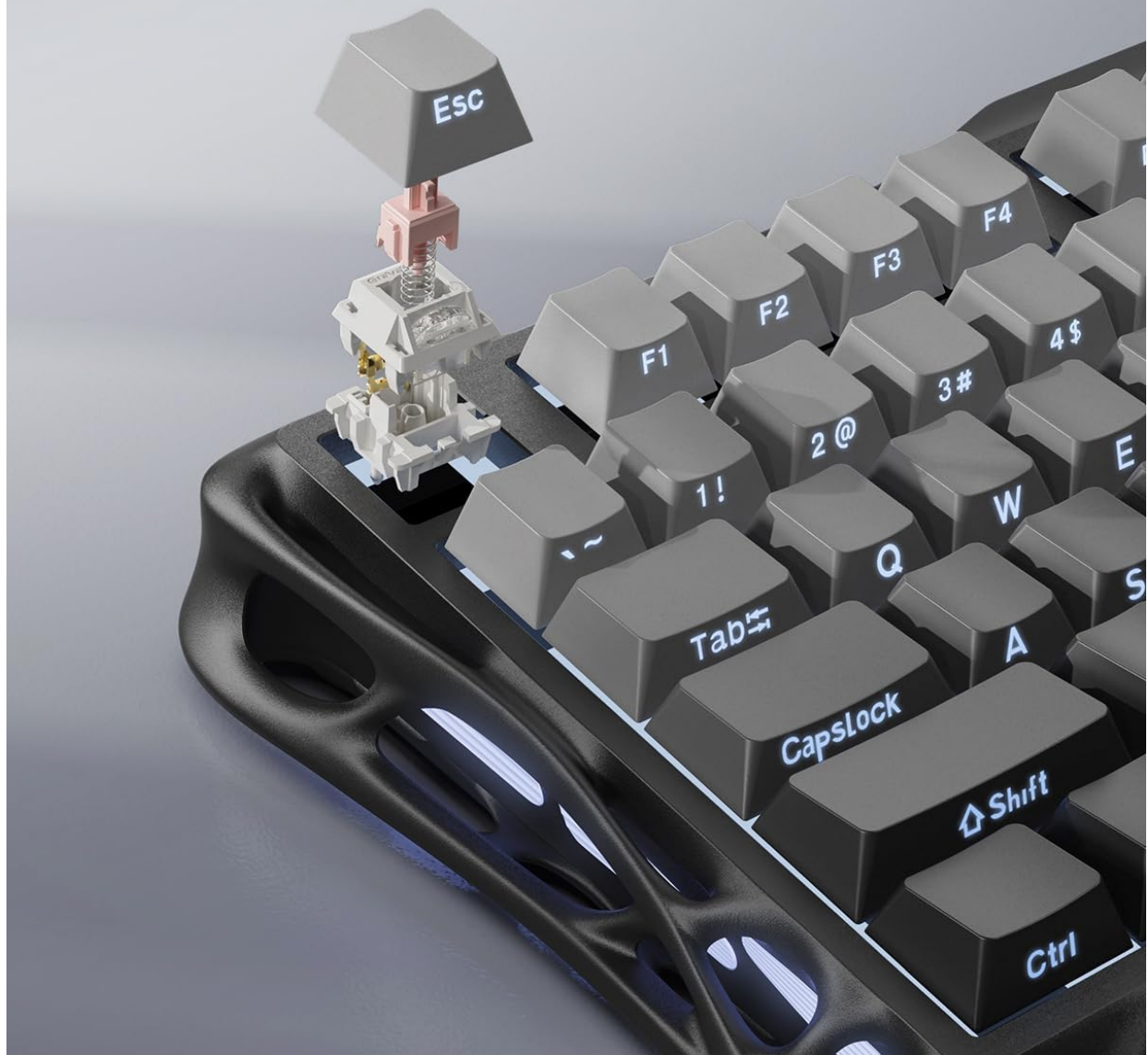
Figure 5.1: Close-up view of the GravaStar Mercury K1's hot-swappable PCB, illustrating a removed keycap and the underlying GravaStar x Kailh Linear switch. This design allows for easy switch replacement.
