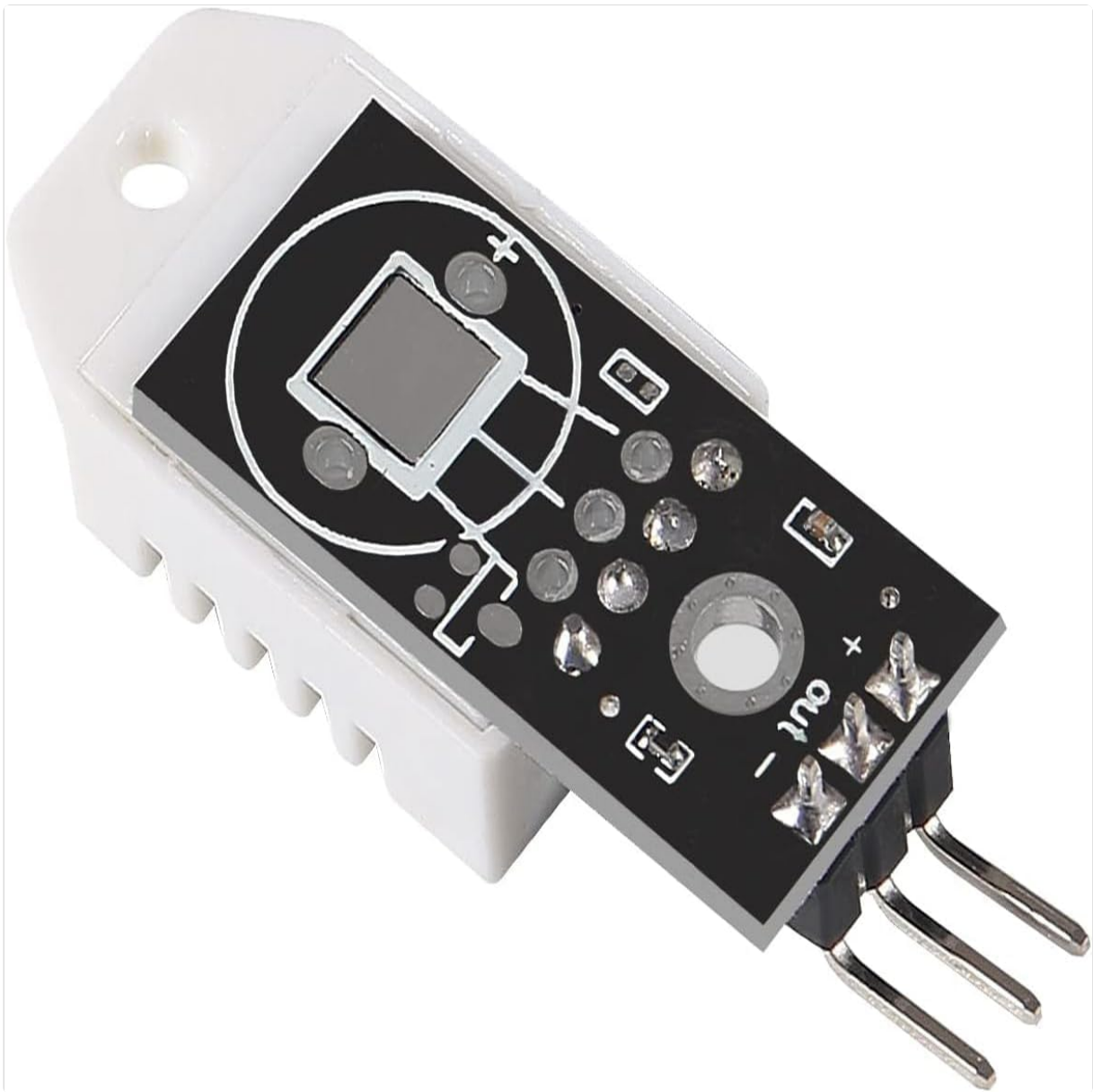
Figure 2: Close-up view of the sensor module's 3-pin interface for wiring.
