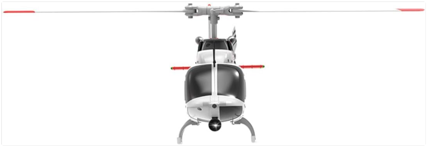
Image: A front view of the helicopter, clearly showing the optical flow sensor mounted on its underside.
