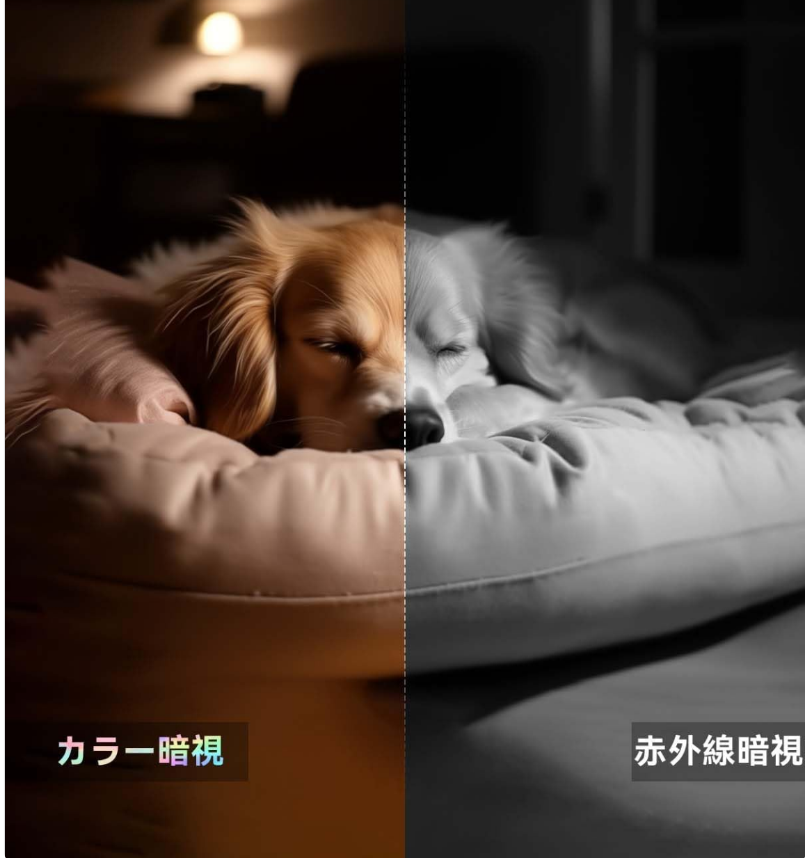
Figure 7: Comparison illustrating the clarity and color retention of full-color night vision versus standard infrared night vision.
