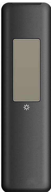
Figure 3.1: Charging options - Solar panel for ambient light charging and USB-C port for cable charging.
