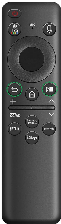
Figure 2.1: Easy setup - Press and hold the Return and Play/Pause buttons for 3 seconds to pair the remote.
