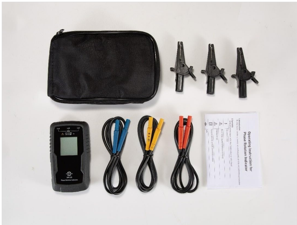
Figure 3.5: All items included with the Spartna SPR-231: the indicator unit, three test leads with alligator clips, and a soft carrying case.
