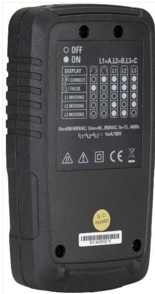
Figure 3.2: Back view of the Spartna SPR-231, illustrating the display legend for phase status and rotation, along with safety markings.
