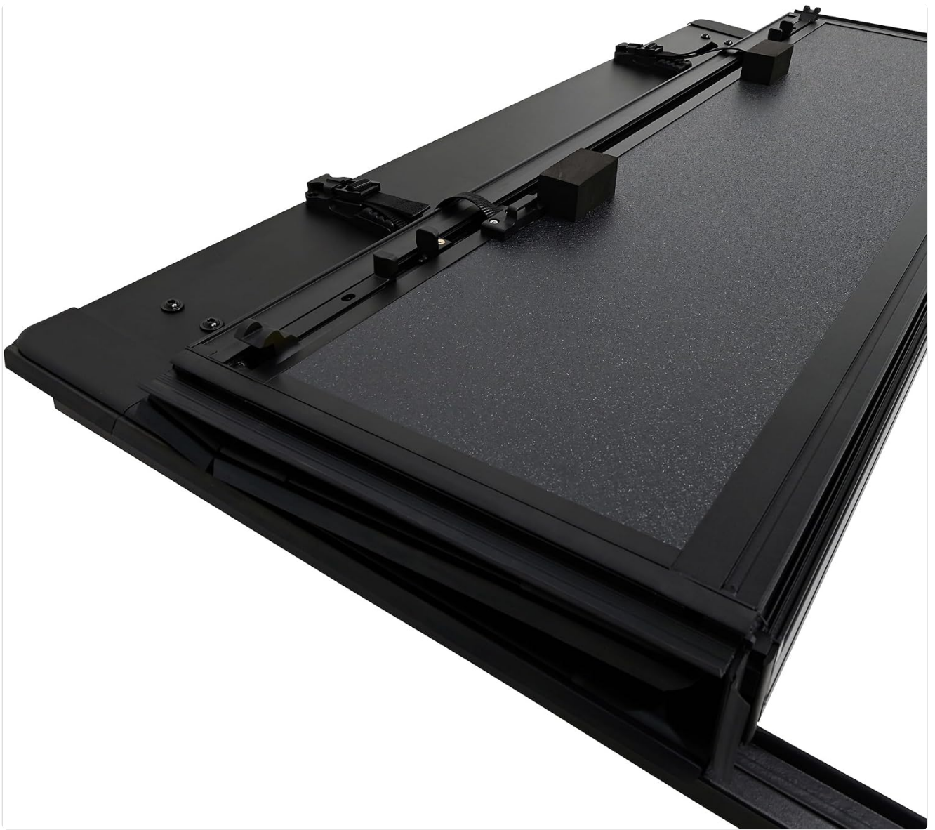
Image: A close-up view of the locking mechanism on the Westin Tri-Fold Tonneau Cover, demonstrating how it secures to the truck bed rail.
