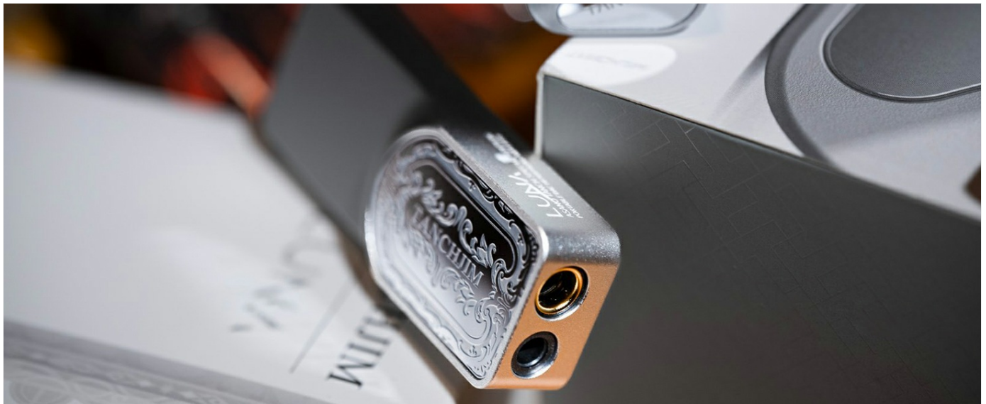
Image 6: LUNA with 3.5mm and 4.4mm output jacks
