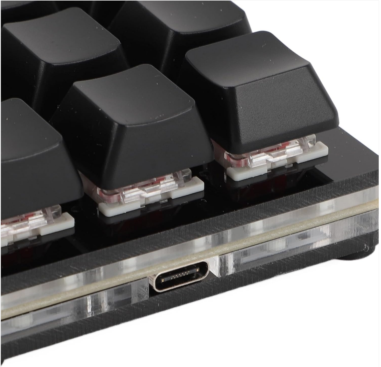
Image: Close-up view of the Type-C USB port located on the side of the keyboard for connection.
