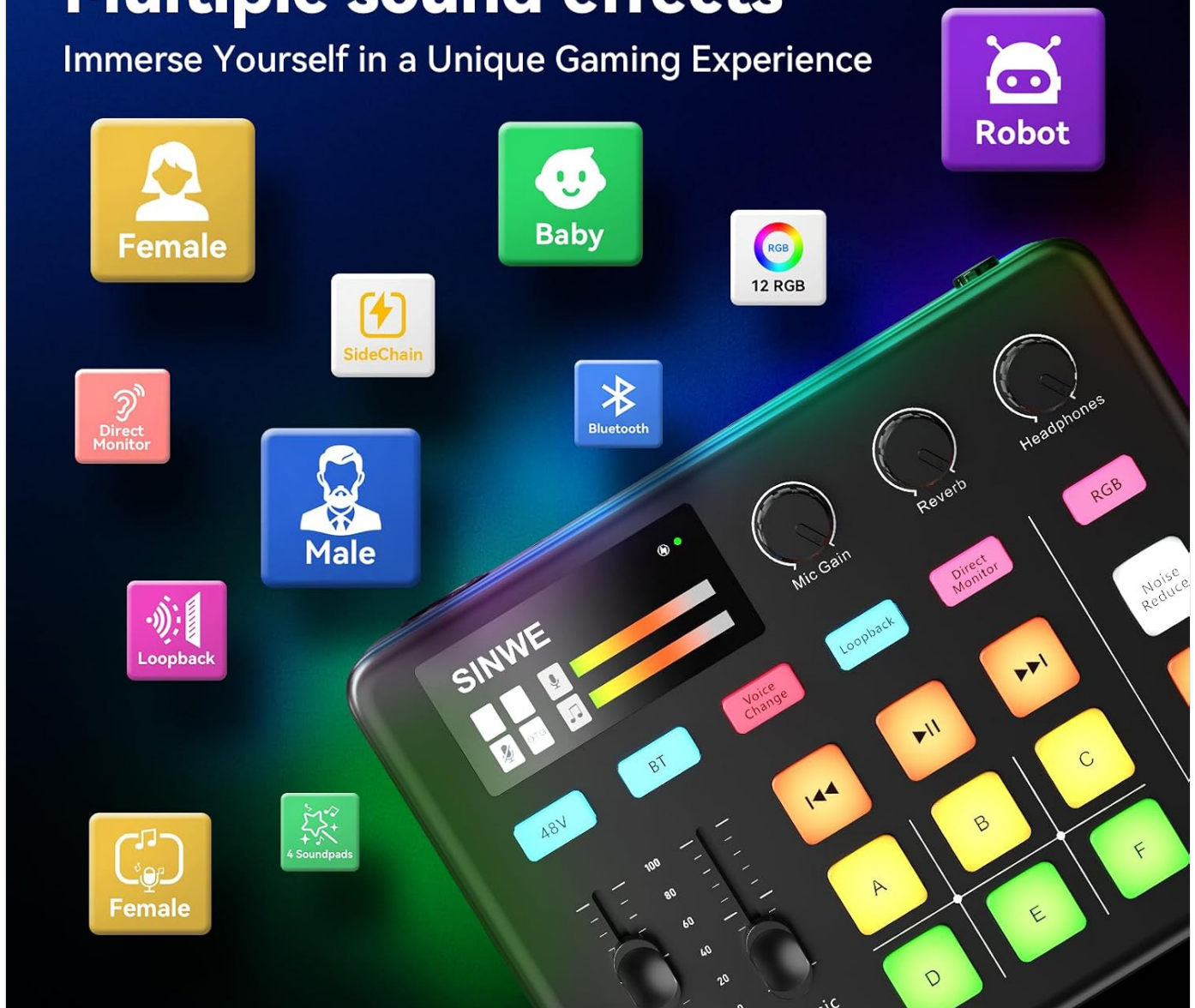
Figure 6.1: The SINWE G1's interface showing the voice changer options (Female, Baby, Male, Robot) and customizable sound pads for various effects.
