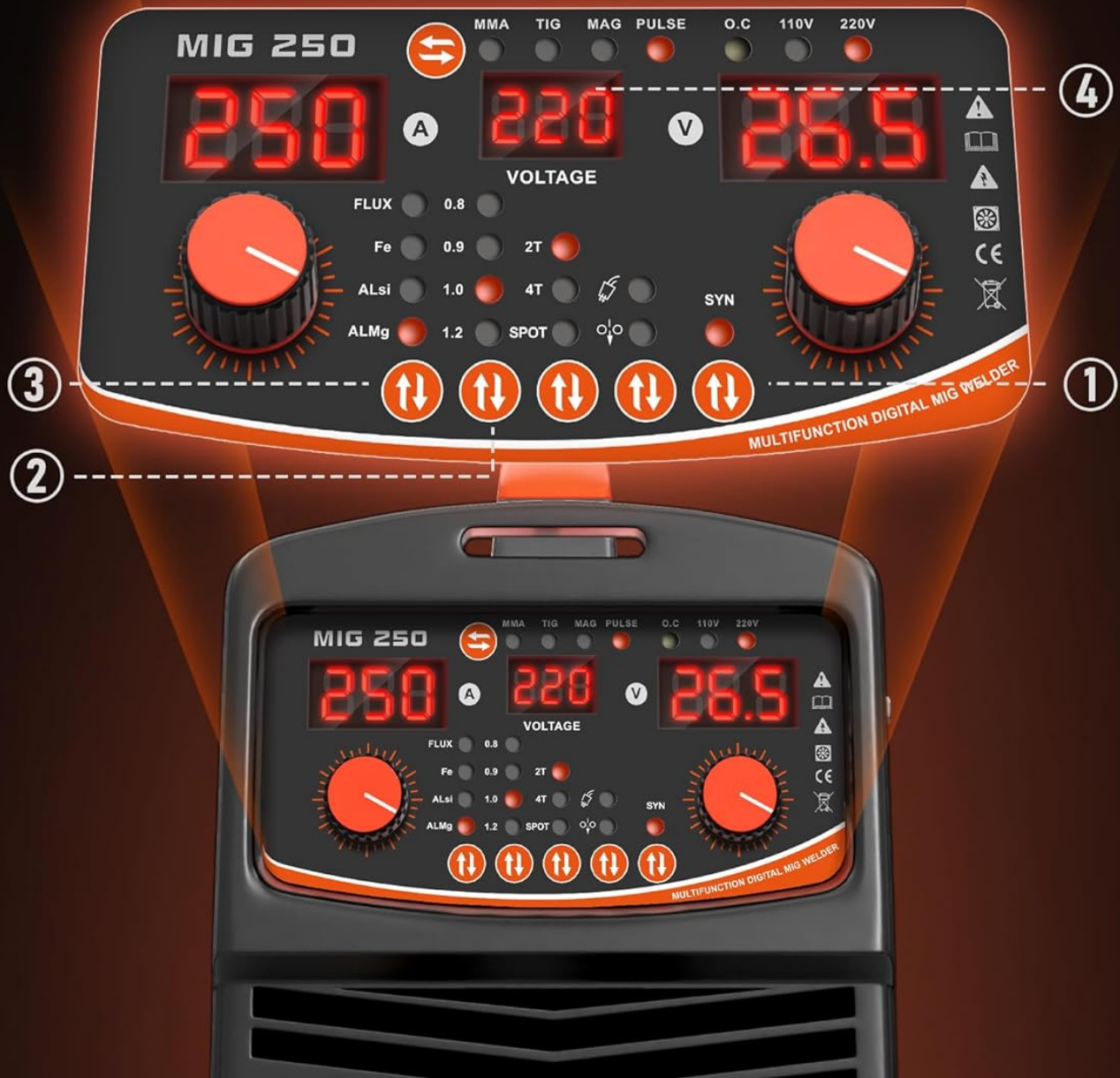
Figure 3.2: Synergic MIG Welding Control Panel.
