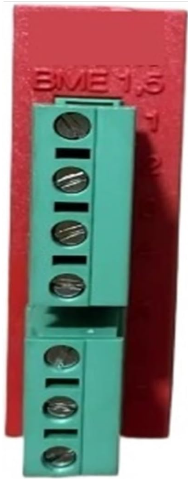
Figure 3.2: Side view of the module, showing the two green terminal blocks where electrical connections are made. The compact nature of the module is evident.
