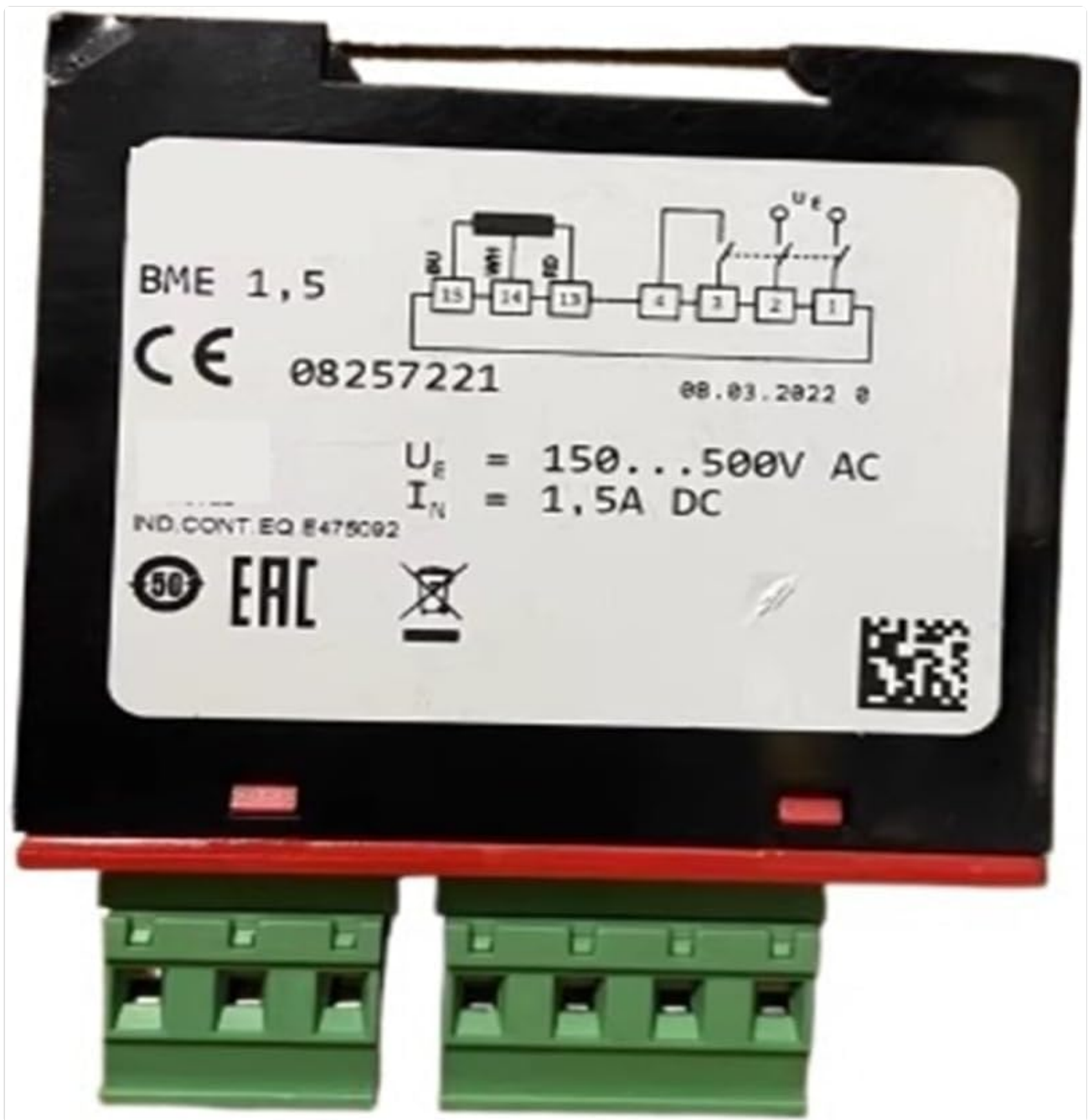
Figure 3.1: Front view of the Aoleaby Motor Brake Rectifier Module BME1.5 08257221. The label displays the model number, CE marking, and electrical specifications including input voltage ( U_e = 150\text{--}500\text{V AC} ) and nominal current ( I_N = 1.5\text{A DC} ). A basic connection diagram is also visible.
