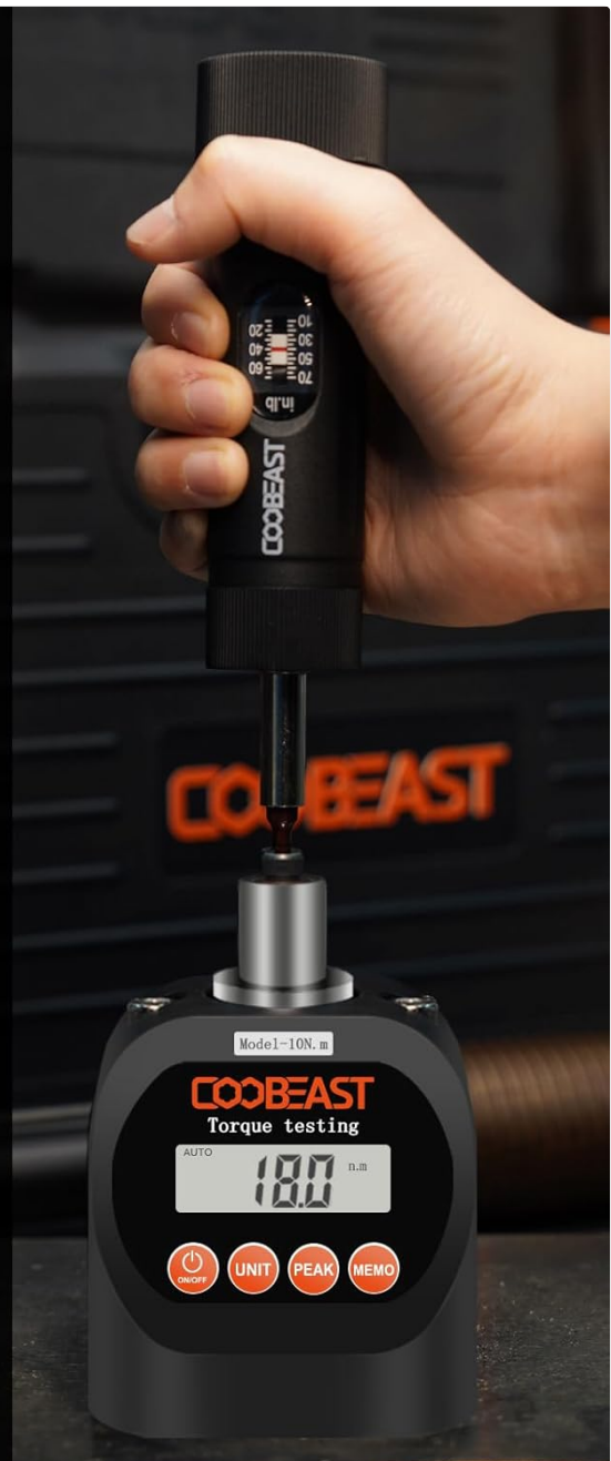
Figure 5: The "click" sound signal indicates reaching the preset torque.
