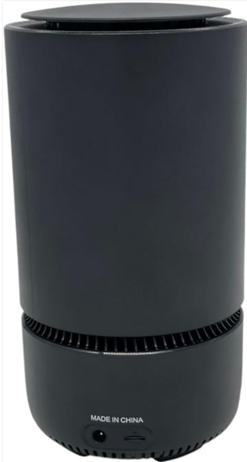
Figure 2: Rear view of the ZAIN-Greenpacket 5G CPE E5-250MK, showing the power input and SIM card slot.
