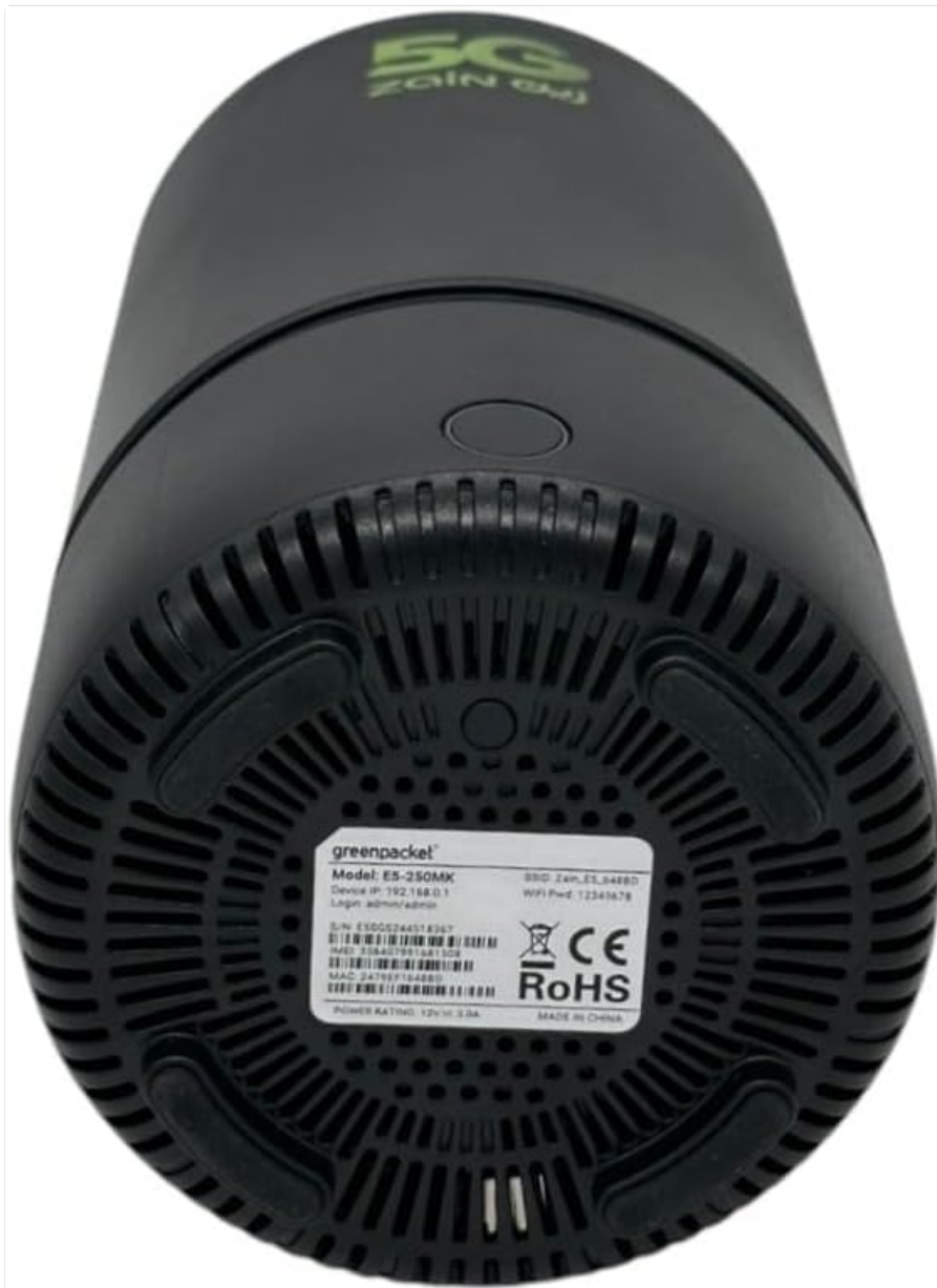
Figure 3: Bottom view of the ZAIN-Greenpacket 5G CPE E5-250MK, showing the product label with model number, default Wi-Fi SSID, password, and power rating.
