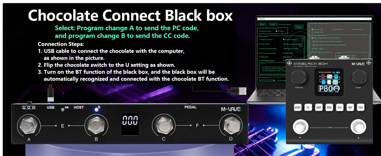
Image: A visual guide demonstrating the two primary connection methods for the M-VAVE Chocolate Plus: wired USB connection to a computer (U mode) and wireless Bluetooth connection to a mobile phone (H mode).
