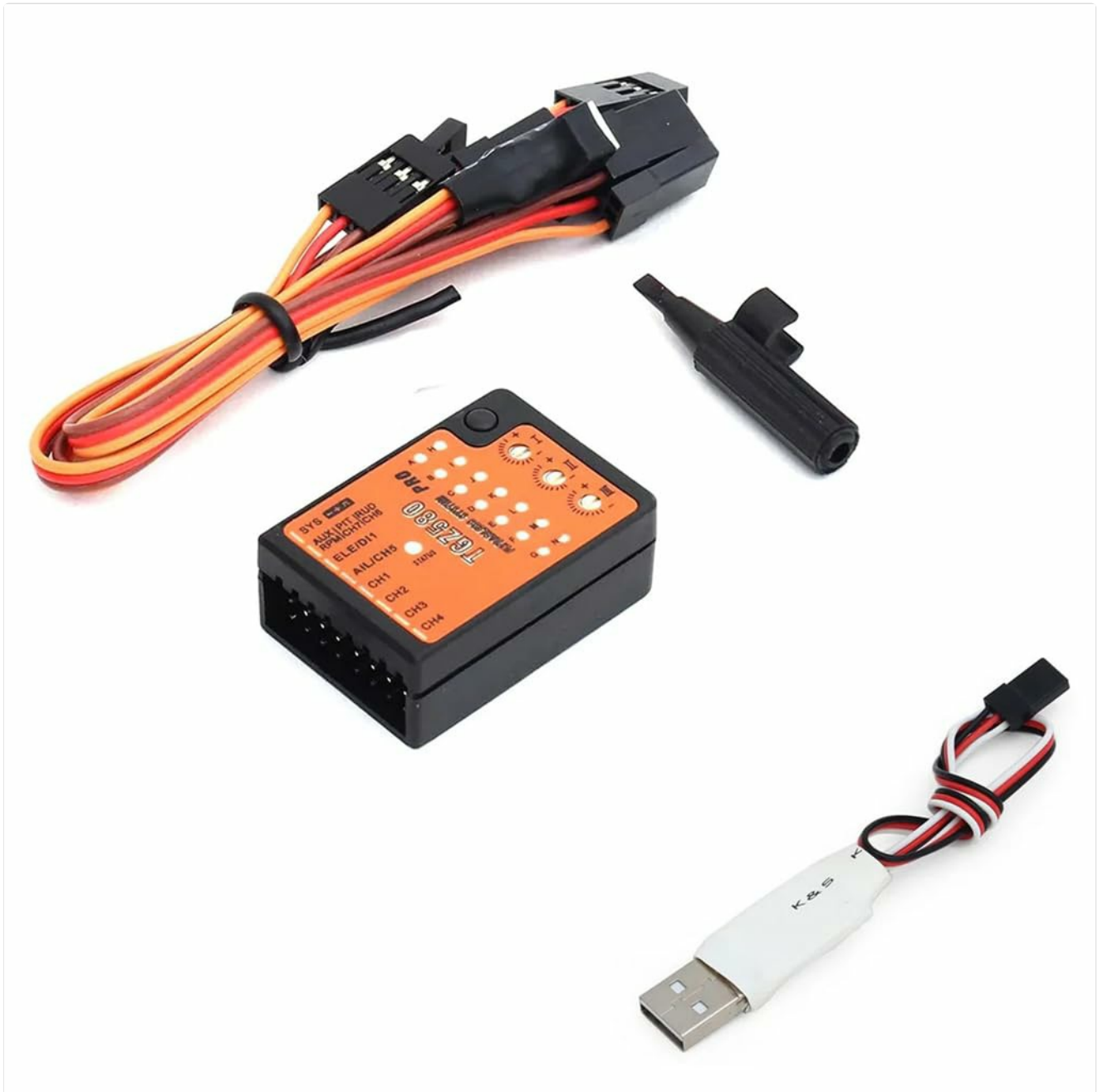
Figure 1: Caruner TGZ580 3-Axis Gyro unit with included wiring harness and USB adapter.
