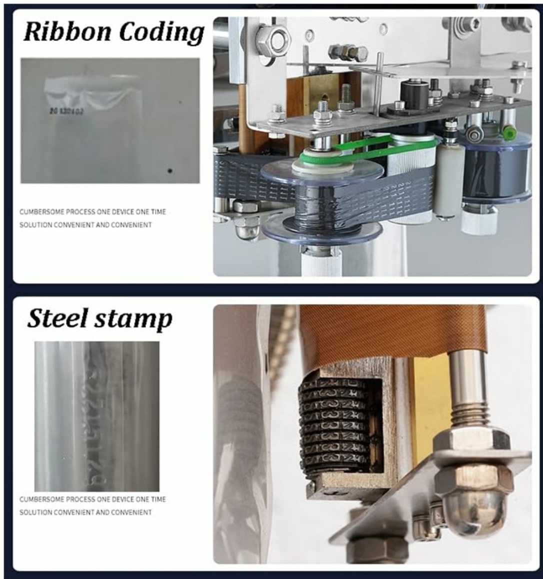
Figure 5.4: Ribbon coding and steel stamp options for batch numbering.
