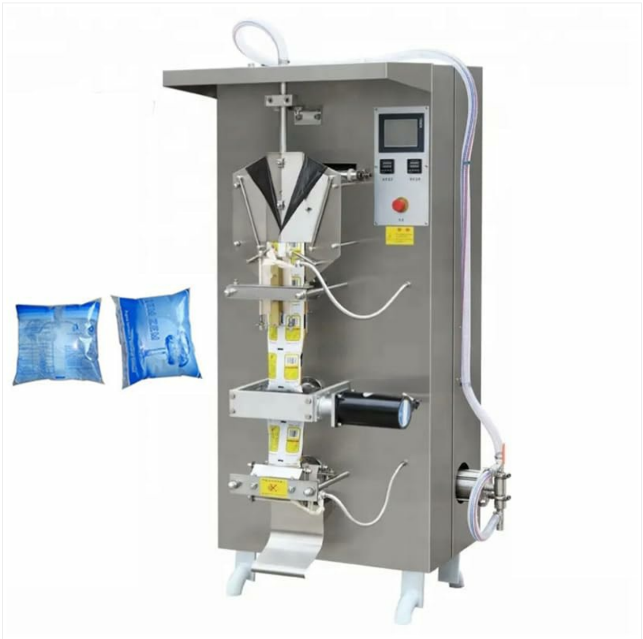
Figure 5.1: The YLZF-1000 machine in operation, producing filled liquid sachets.
