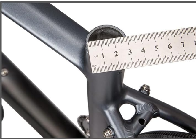
Image 4.1: Visual guide for measuring the diameter of your existing seatpost or the inside diameter of your bike frame's seat tube using a caliper or ruler.
