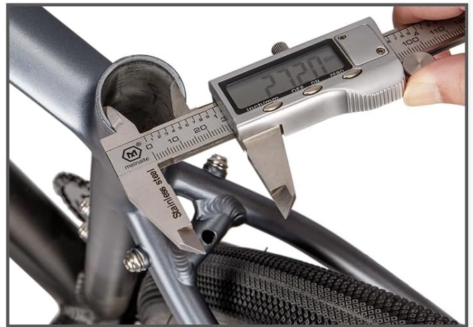
Image 4.1: Visual guide for measuring the diameter of your existing seatpost or the inside diameter of your bike frame's seat tube using a caliper or ruler.
