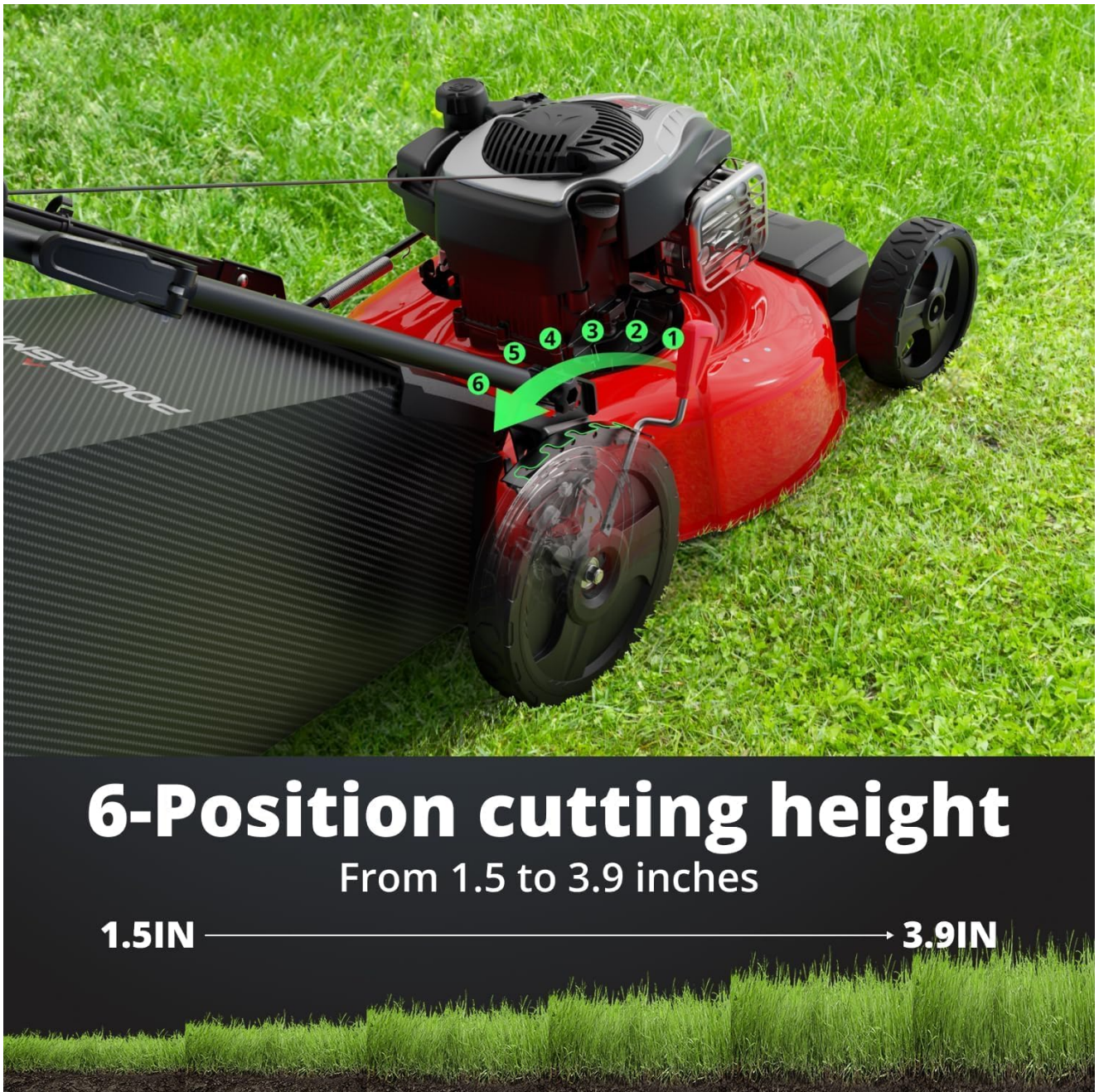
Image 3.2: Height Adjustment. This image illustrates the lever used to adjust the cutting height, with indicators for different settings.
