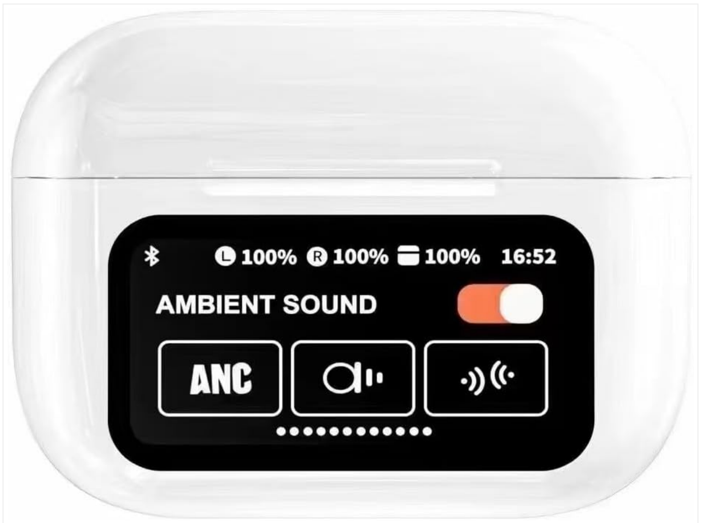
Image 1: A9PRO Wireless Earbuds Charging Case Display. The display shows battery levels for the left earbud (L 100%), right earbud (R 100%), and the charging case (100%), along with the current time (16:52). It also indicates "AMBIENT SOUND" with a toggle switch, and three mode buttons: "ANC" (Active Noise Cancellation), an icon for Ambient Sound, and an icon for Normal mode.
