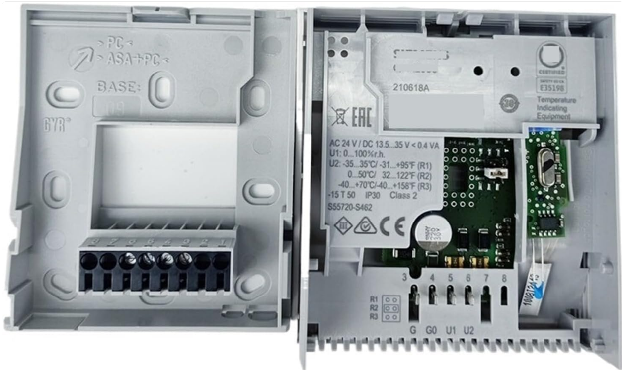
Figure 2: Internal view of the SHHJCO QFA2000 sensor, displaying the terminal block for electrical connections and the main circuit board. The terminals are labeled G, G0, U1, U2.
