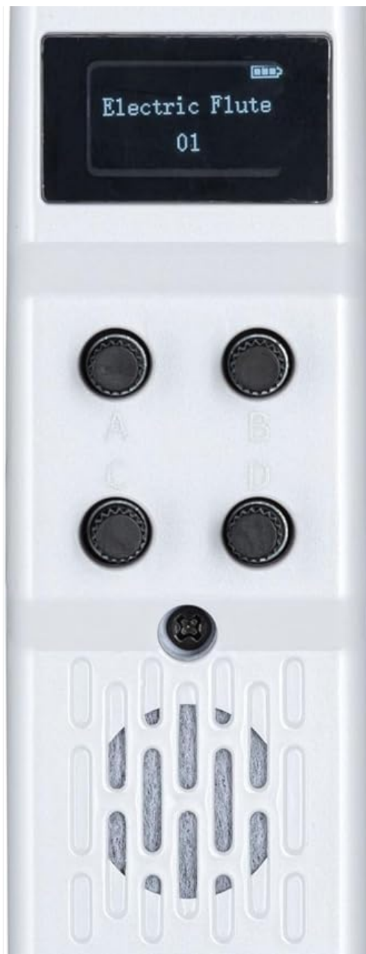
Figure 4.5: Close-up of the display screen and associated control buttons on the upper section of the device, showing instrument selection.
