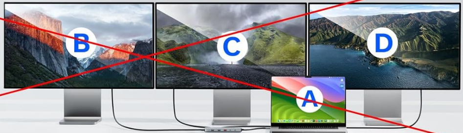
Figure 3: Illustration of triple monitor configurations for macOS systems, highlighting the limitation of extending only one monitor.
