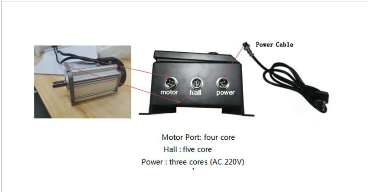
Figure 7: Diagram illustrating the connection ports on the BLDC motor driver. From left to right: Motor Port (four core), Hall Port (five core), and Power Port (three core, for AC 110-130V input).
