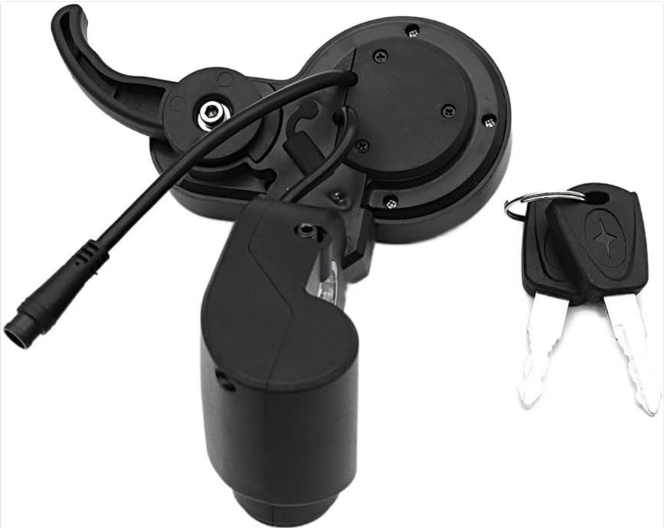
Figure 4.2: The ZQ-100 Mileage Meter with key ignition.
