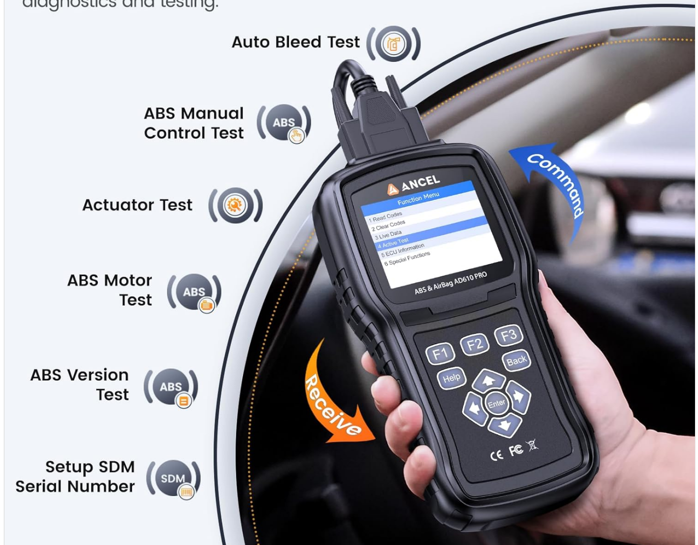
Figure 6: Diagram illustrating the bidirectional control and active test capabilities of the AD610 PRO for ABS/SRS systems, showing commands sent and data received from the vehicle's ECU.
