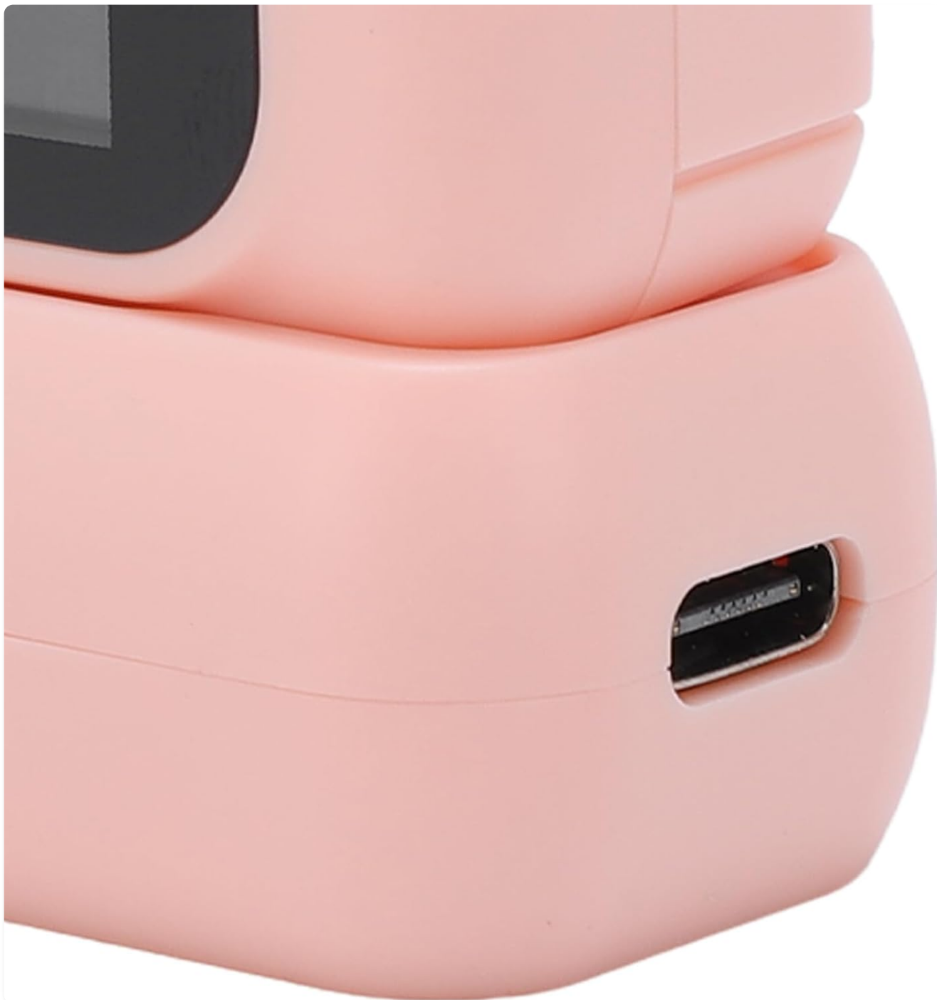
Figure 4: USB-C charging port on the detachable base.
