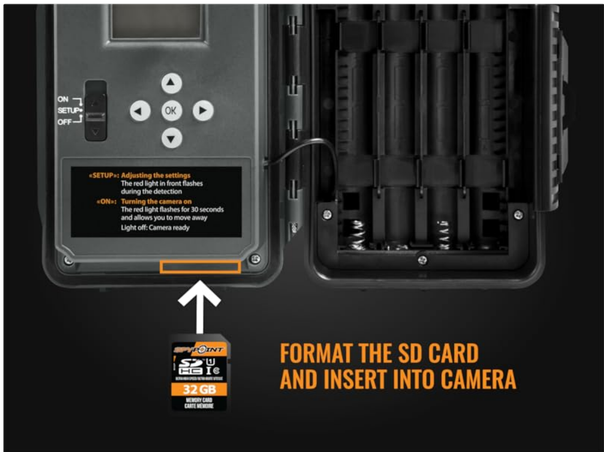
Image: Instructions for inserting an SD card and formatting it using the camera's internal menu.
