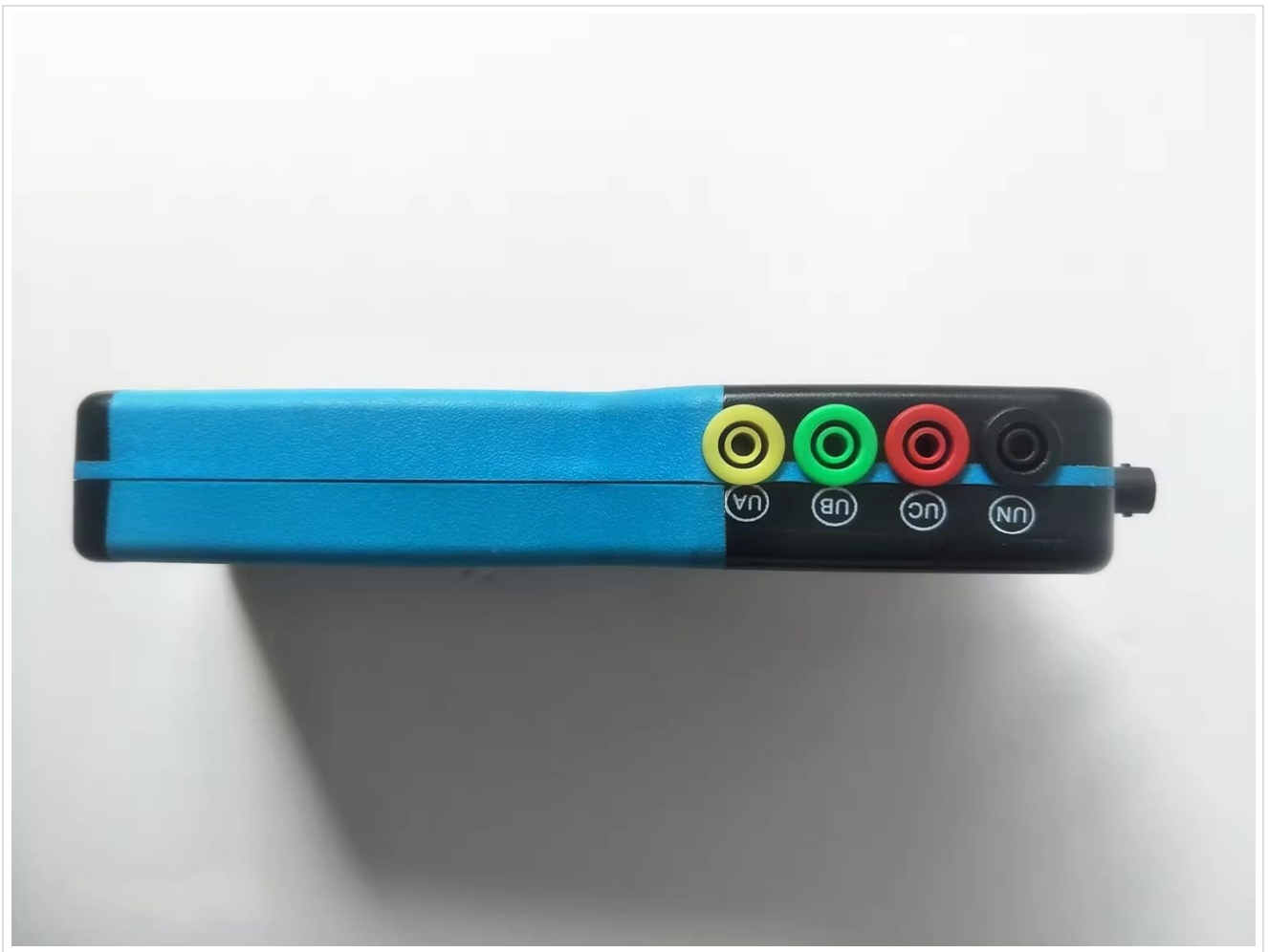
Figure 4: Side view of the ME435 unit displaying the various input jacks for measurement connections.
