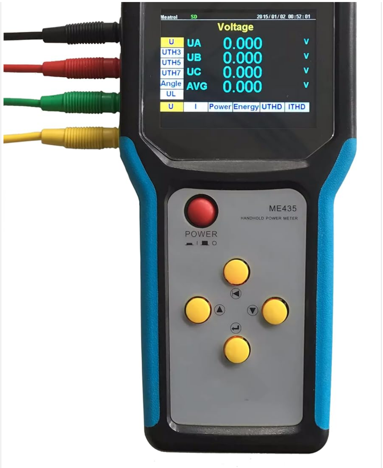
Figure 3: Rogowski coils connected to the top input ports of the ME435 unit.
