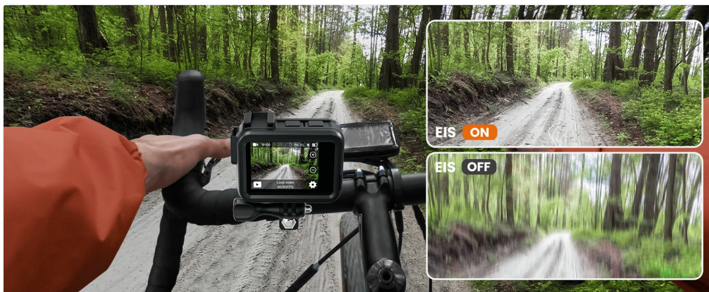
Image: A side-by-side comparison of video footage, demonstrating the effect of Electronic Image Stabilization (EIS) when turned on versus
