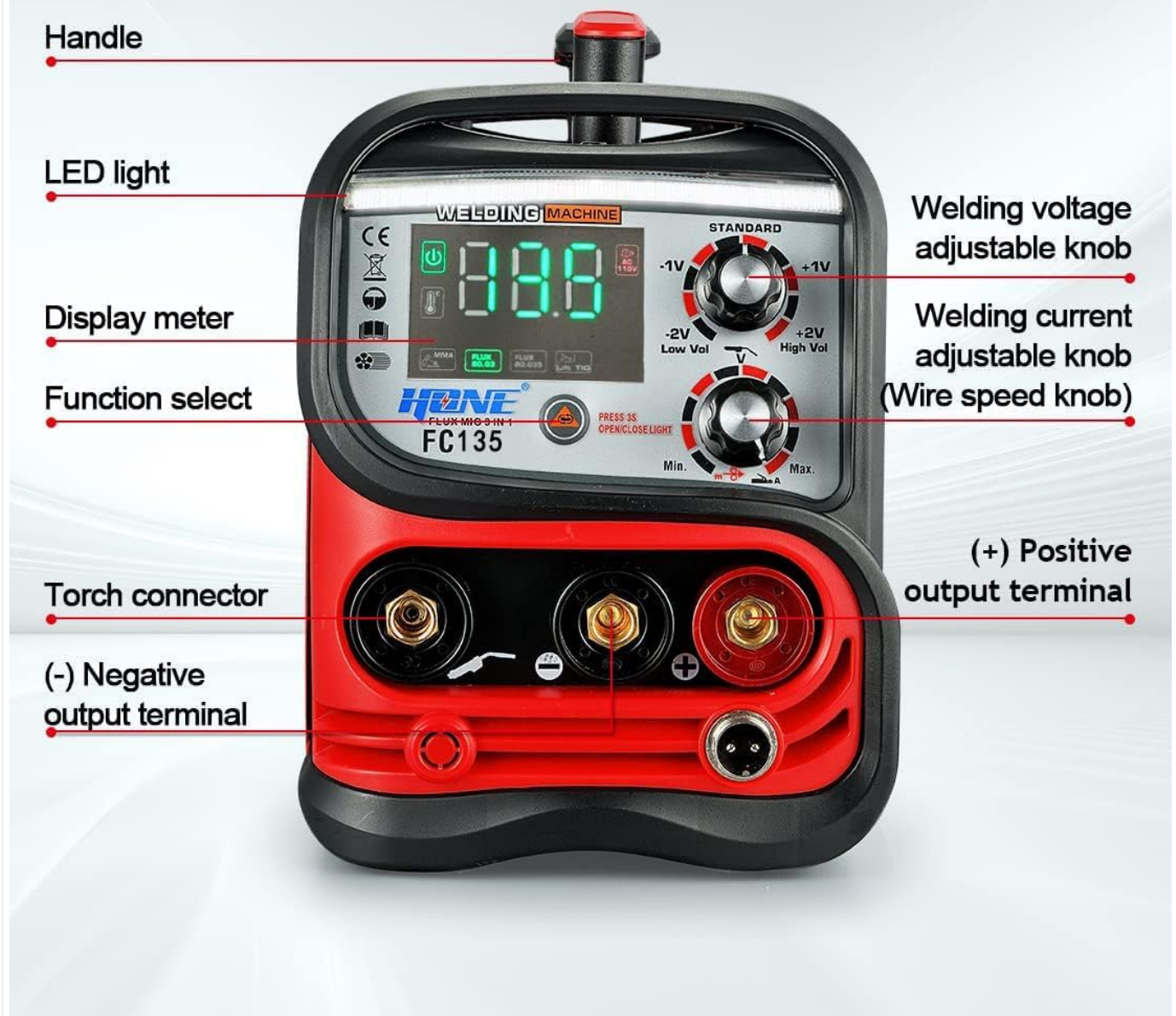
Figure 4.1: Front panel layout and controls of the HONE FC135.
