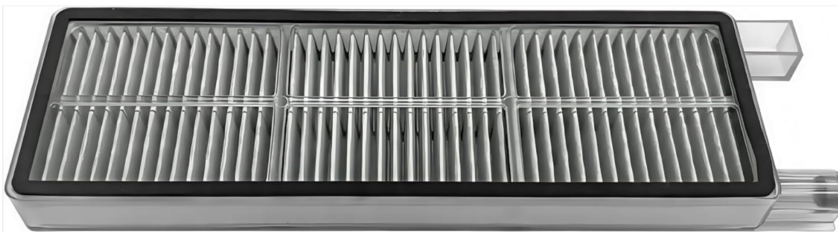
Figure 4.4: A close-up of the high-efficiency particulate filter, designed to capture 99.97% of particles as small as 0.3 microns.
