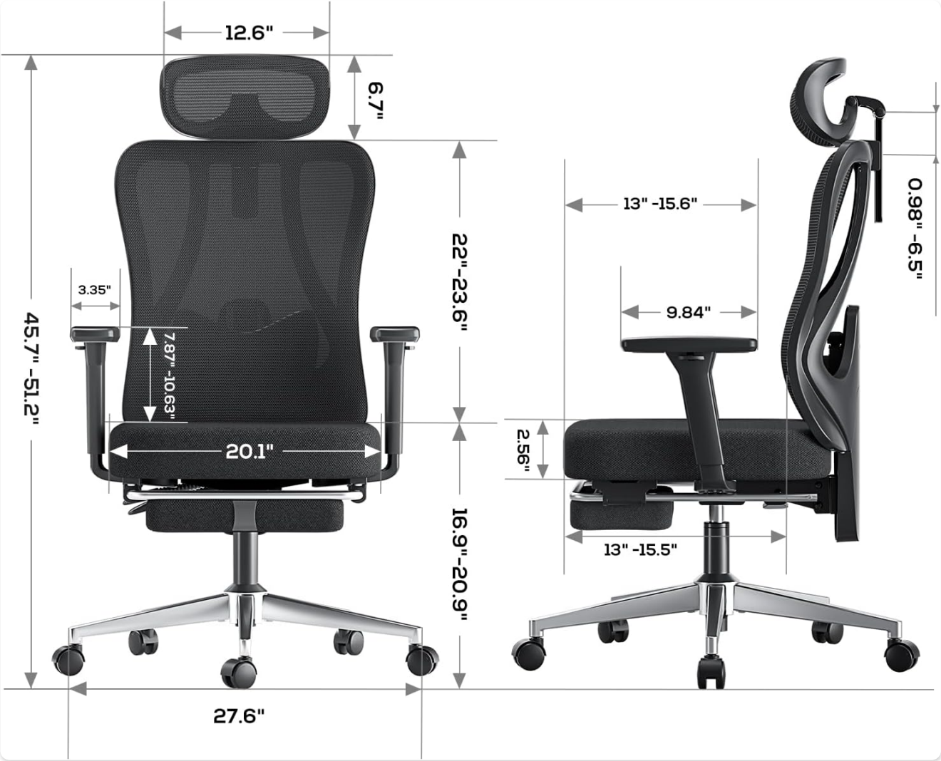
Figure 2: Detailed dimensions of the Hbada P3 Pro Office Chair.
