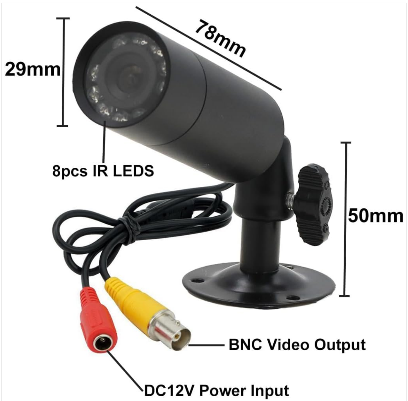
Figure 6.2: Camera dimensions and port identification. The camera body is approximately 78mm long and 29mm in diameter, with a total height of 50mm including the bracket. It features 8 IR LEDs, a BNC video output, and a DC12V power input.
