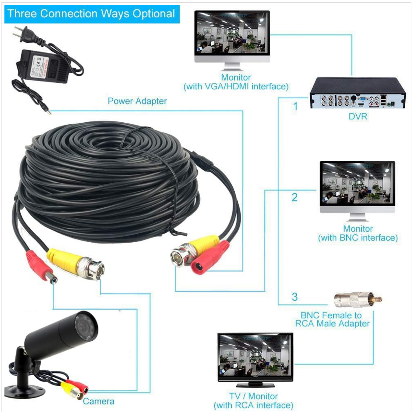
Figure 6.3: Three optional connection methods for the camera. The camera connects to a power adapter (DC12V) and an extension cable for video. The video signal can then be connected to a DVR, a BNC-compatible monitor, or an RCA-compatible TV/monitor via an adapter.
