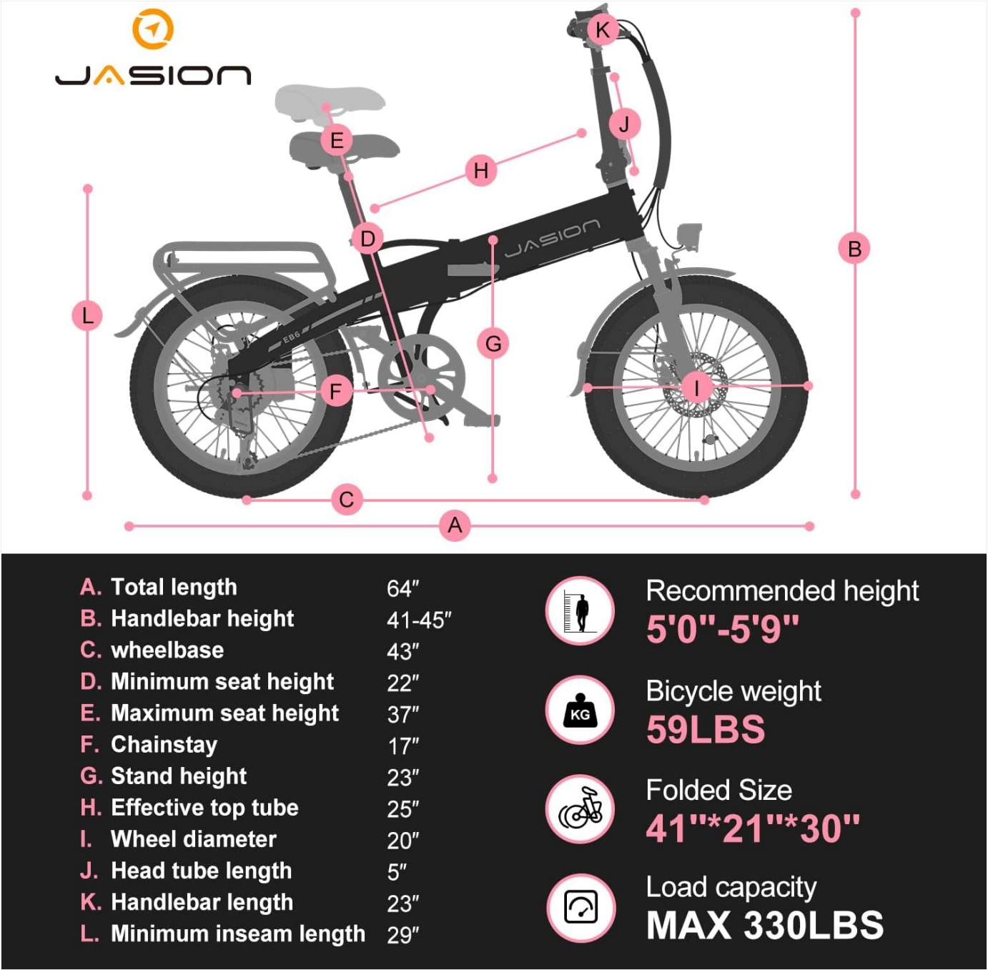
Image: Jasion EB6 Electric Bike dimensions, including total length, handlebar height, wheelbase, seat heights, wheel diameter, and recommended rider height (5'0"-5'9").
