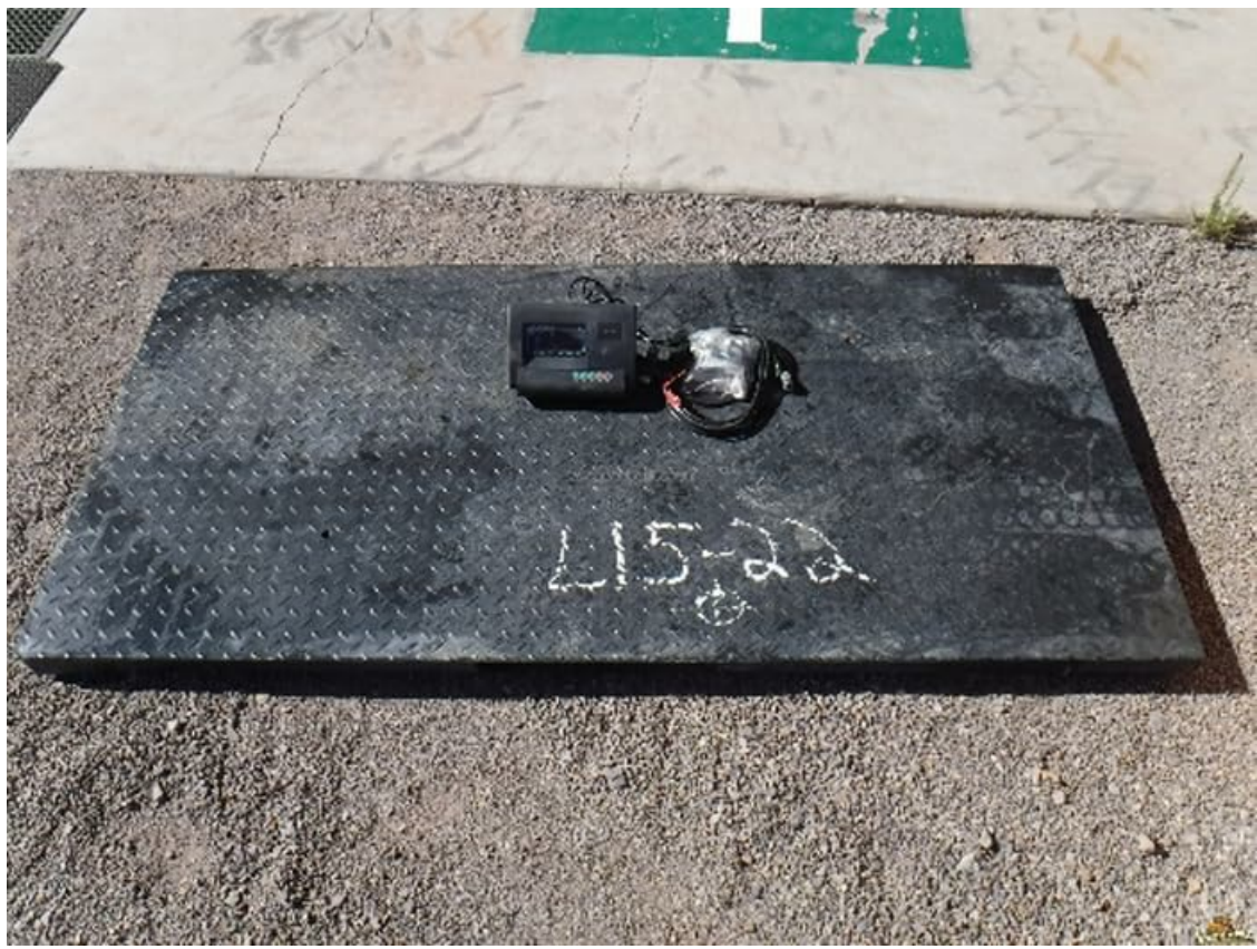
Image 3.2: The XK3190 A12E indicator connected to a large industrial floor scale, showing its application versatility.
