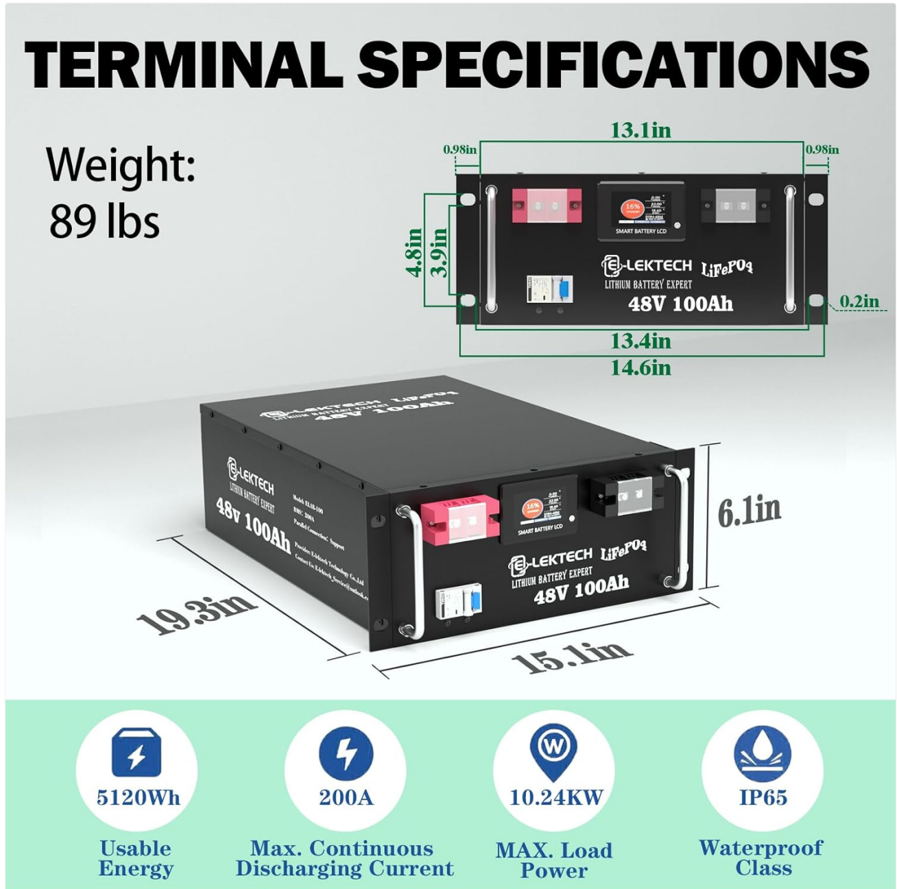
Figure 3: Detailed dimensions and terminal specifications for installation planning.
