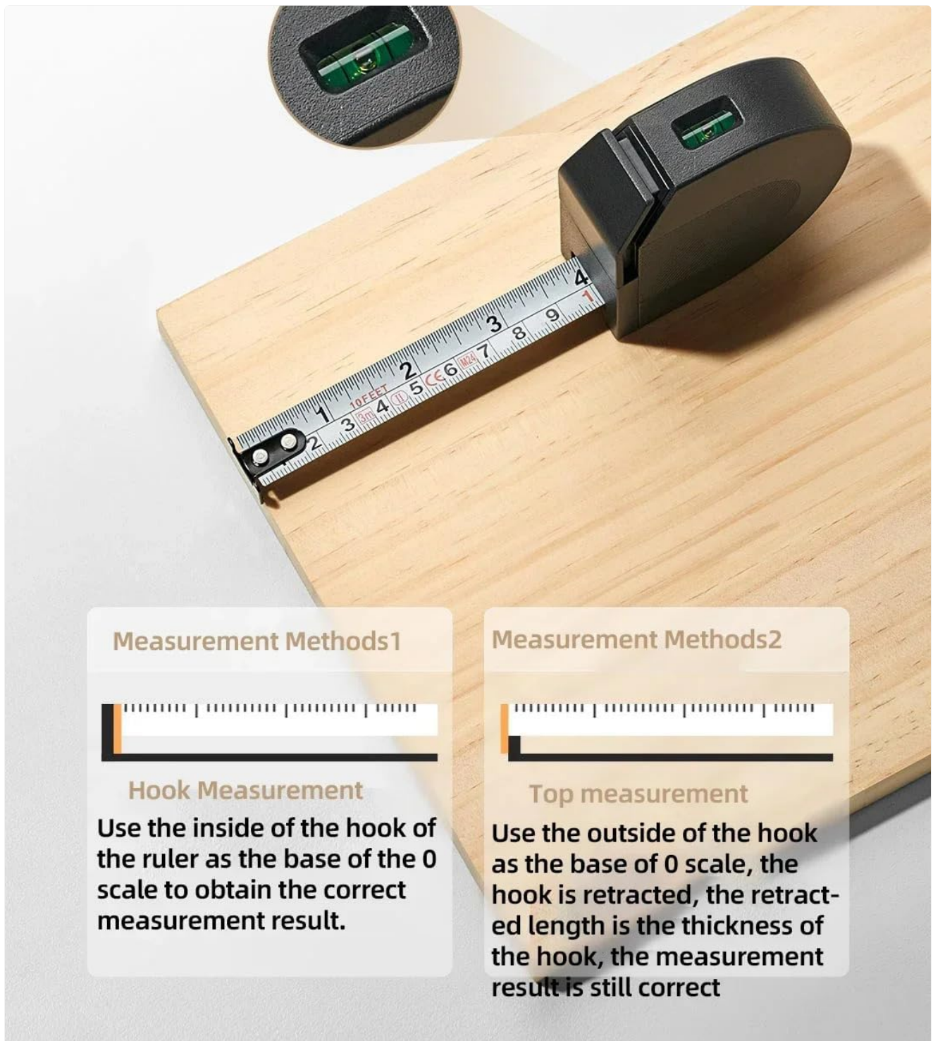
Figure 4.4: The self-locking tape measure with integrated level and different measurement techniques.
