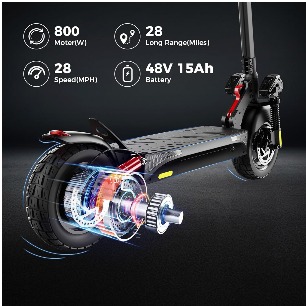
Figure 2.2: Overview of iX4 motor, range, speed, and battery specifications.
