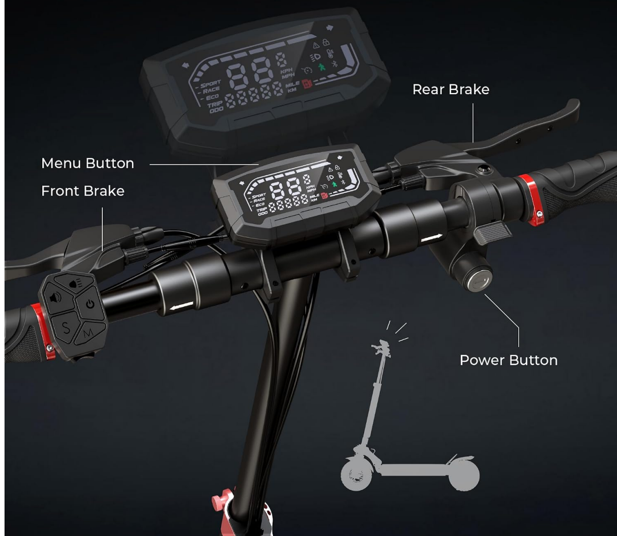
Figure 2.3: Multi-function LED dashboard and controls.
