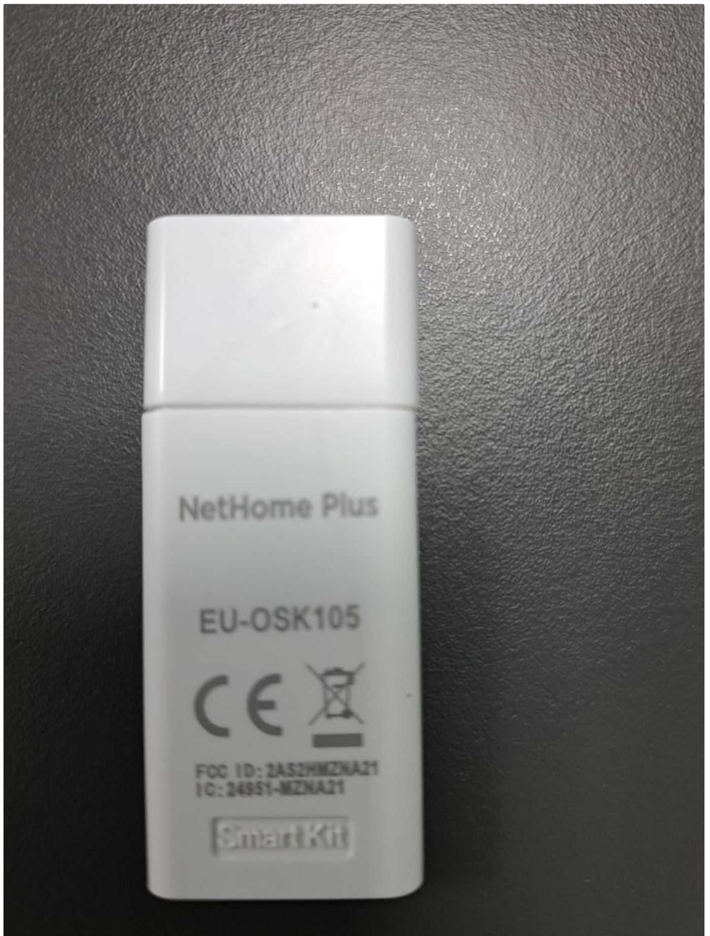
Figure 2: The SMART KIT EU-OSK105 WiFi module with its protective cap in place, displaying 'Smart Kit' and a QR code.
