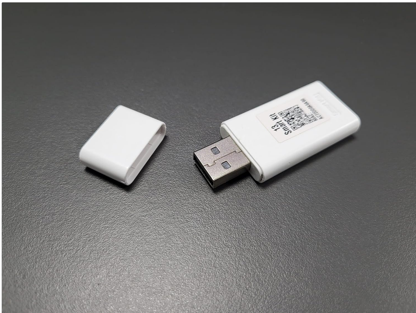
Figure 1: Close-up view of the SMART KIT EU-OSK105 WiFi module, showing 'NetHome Plus EU-OSK105' branding and regulatory markings.
