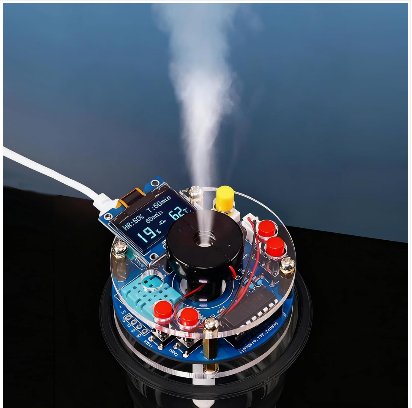
Figure 2: The fully assembled humidifier kit in operation, demonstrating mist output and the OLED display.
