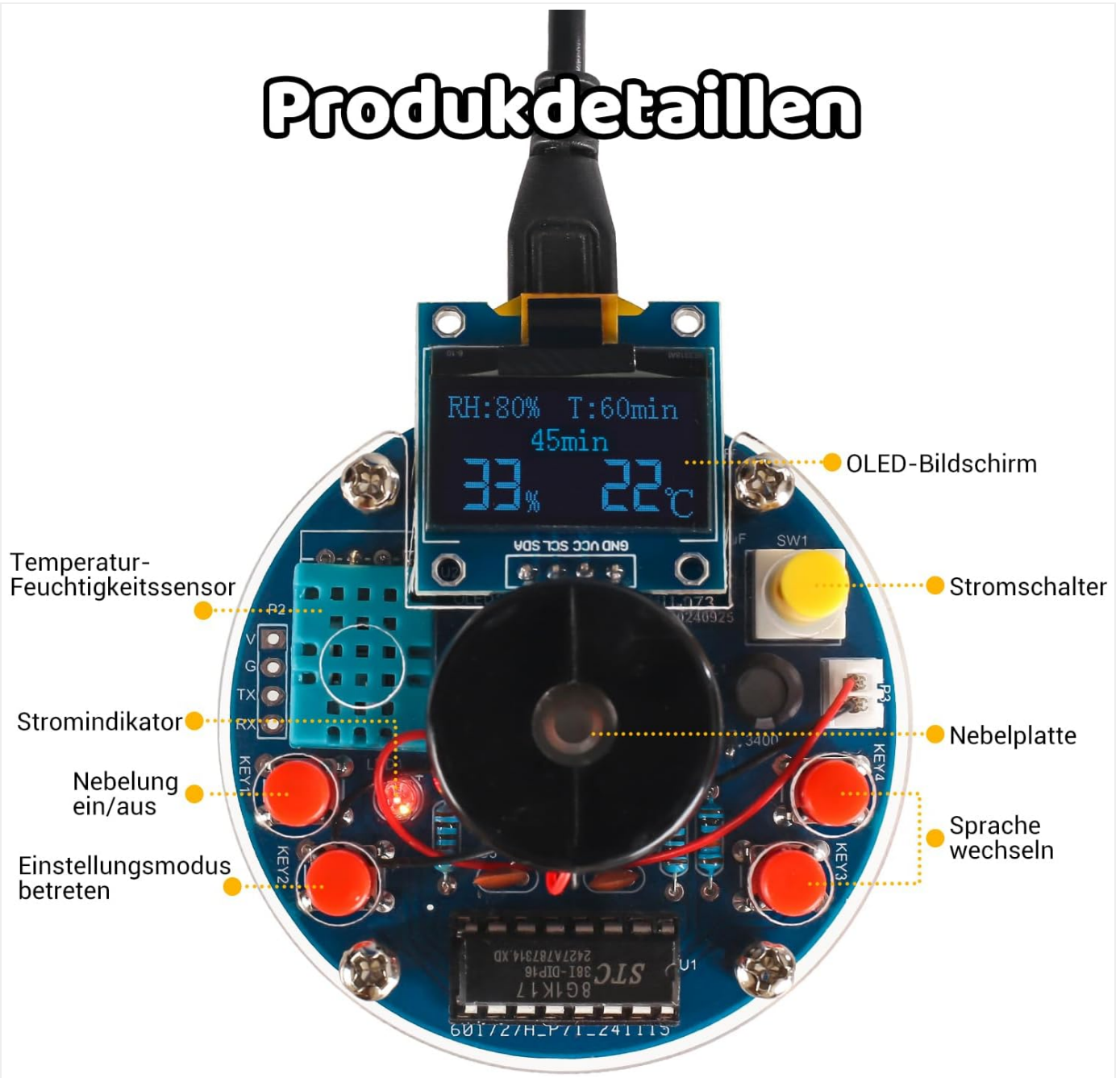
Figure 3: Detailed view of the humidifier's components and controls, including the OLED screen, power switch, nebulizer plate, and control buttons (KEY0, KEY1, KEY2, KEY3).
