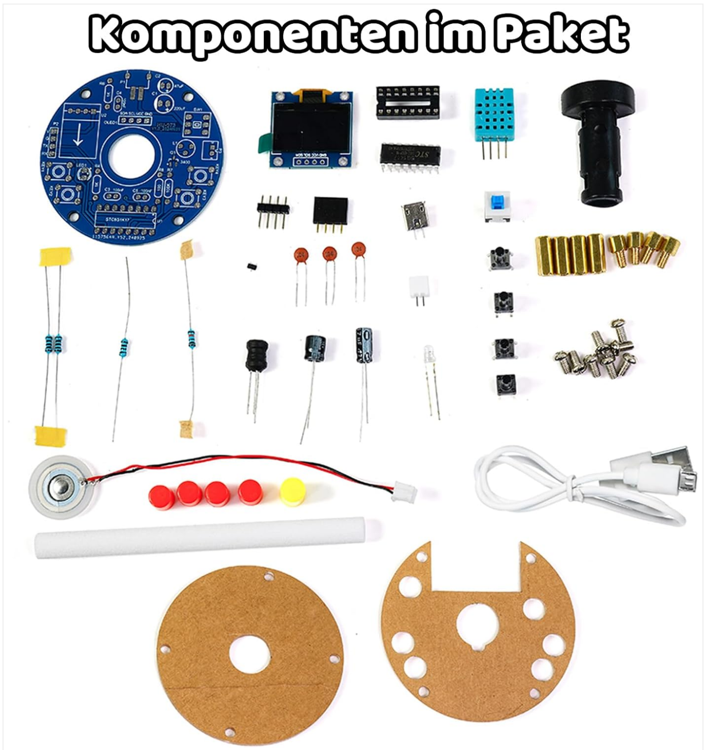
Figure 1: All components included in the BANRIA DIY Soldering Kit Humidifier package. This includes the main PCB, OLED display, various resistors, capacitors, buttons, sensors, a nebulizer, USB cable, and acrylic casing parts.
