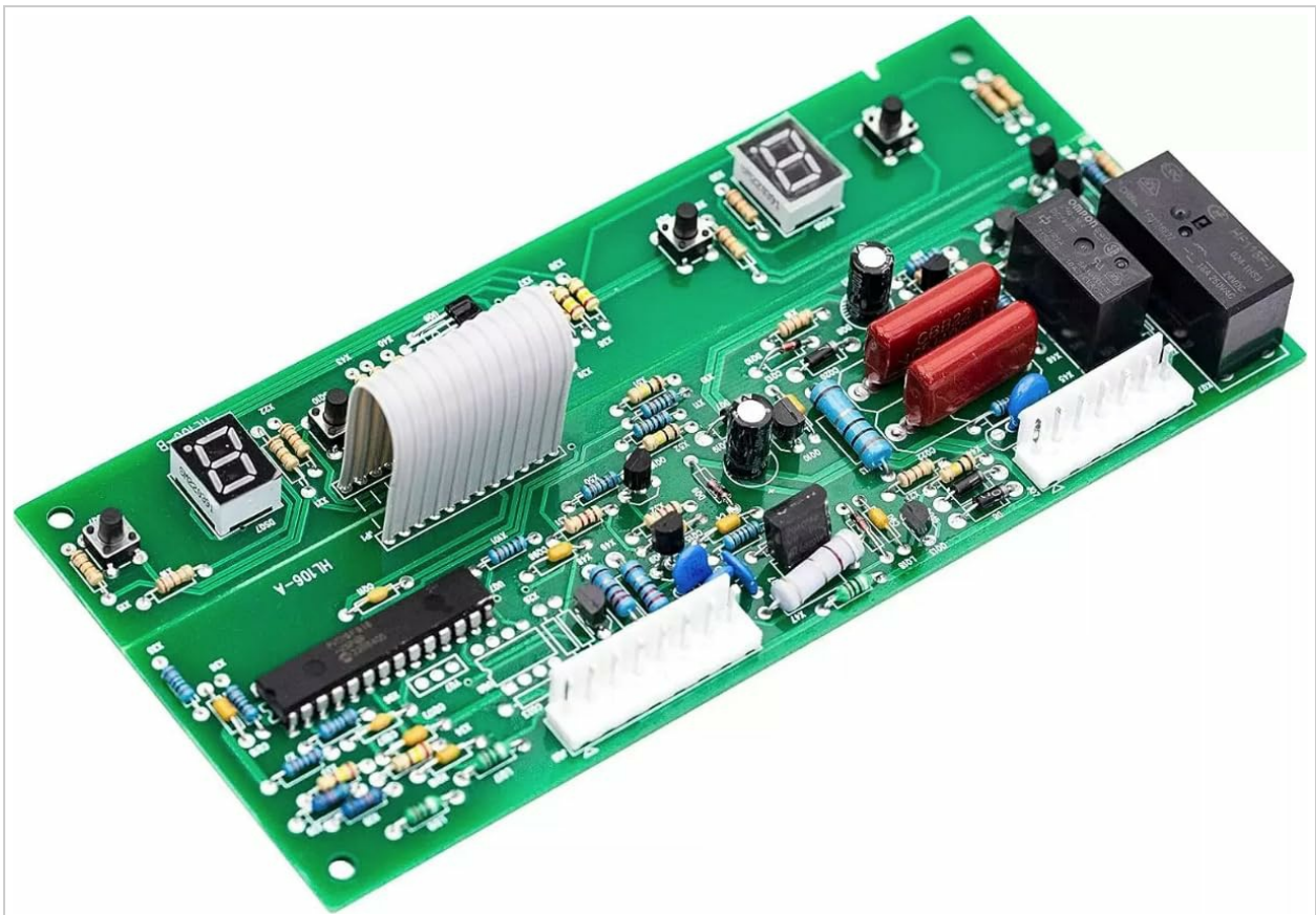
Image 1.1: Generic Replacement Control Board. This image displays the replacement control board, showing its connectors and electronic components. It is designed to replace the original control board in compatible refrigerator models.
