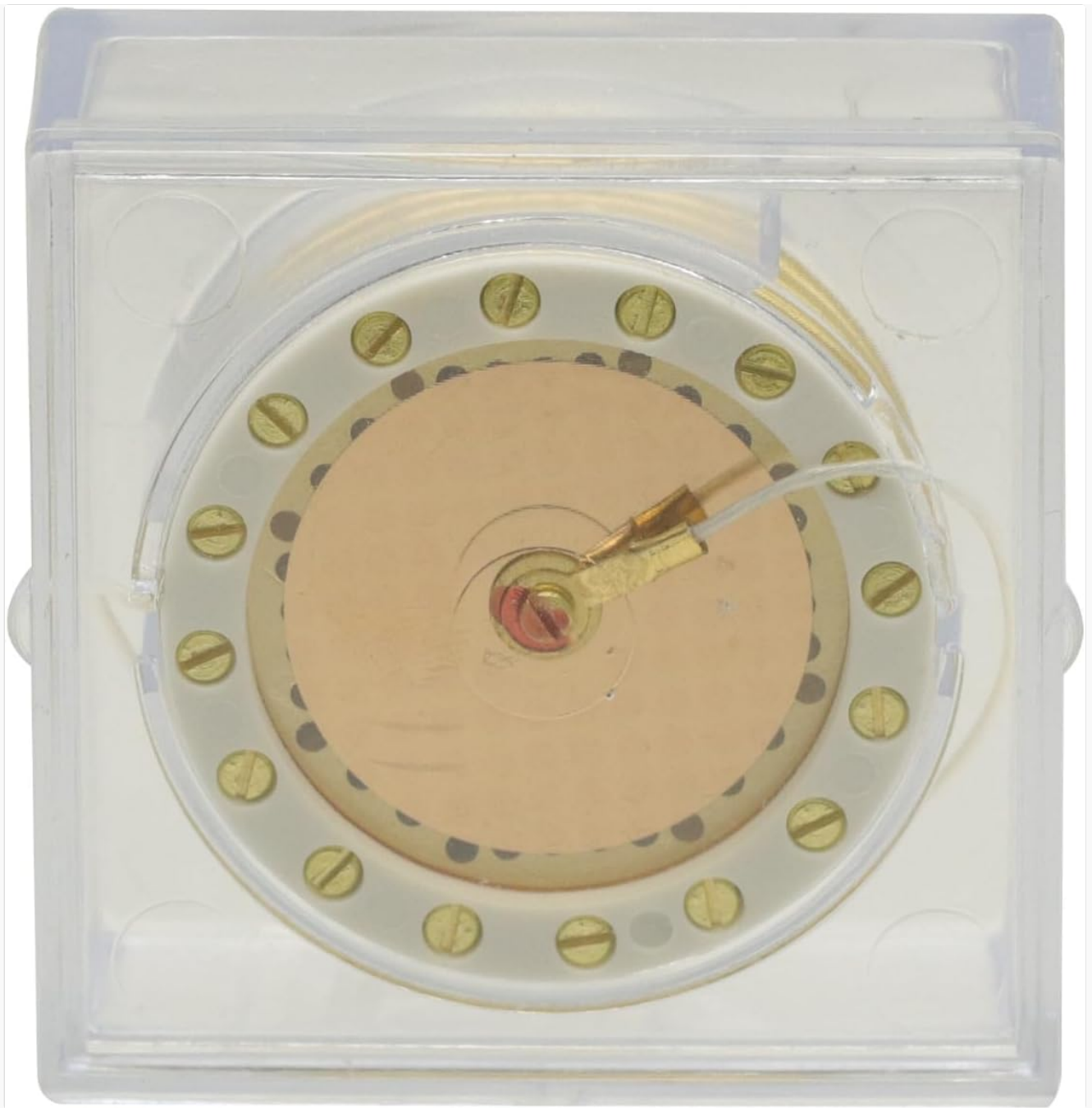
Figure 4: The RK-87 diaphragm housed in a clear protective case, illustrating its delicate nature.
