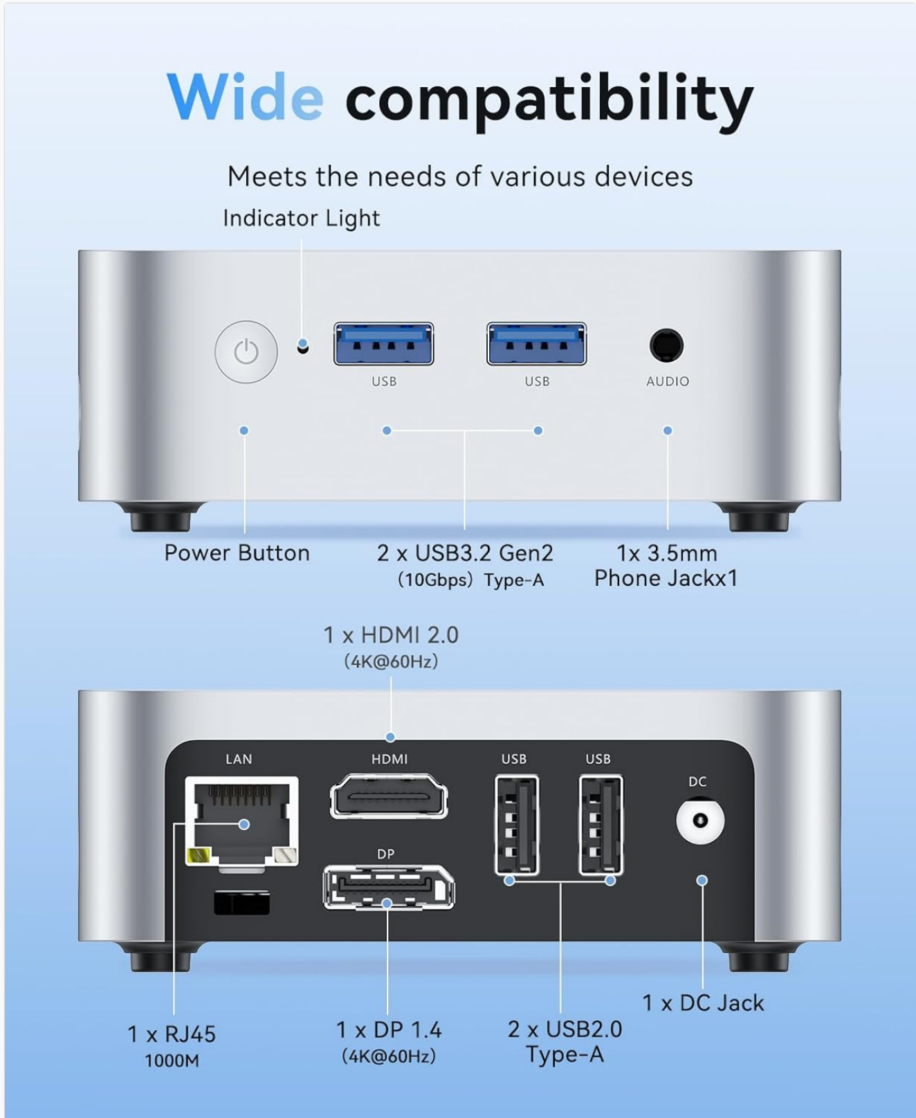
Figure 3.1: Front and Rear Ports of the ACEMAGIC Vista Mini V1. The top part of the image shows the front panel with a power
