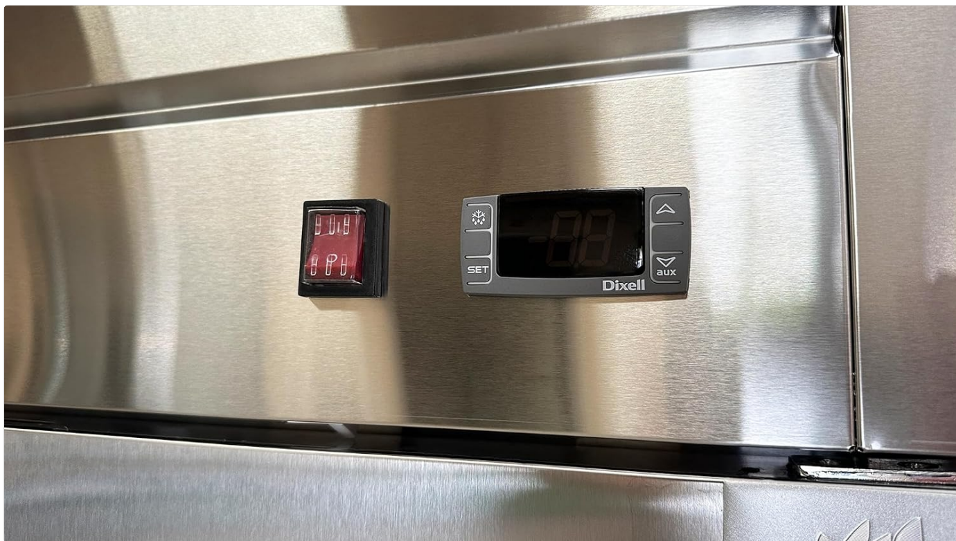
Figure 4: Close-up of the digital temperature control panel (Dixell) and power switch.
