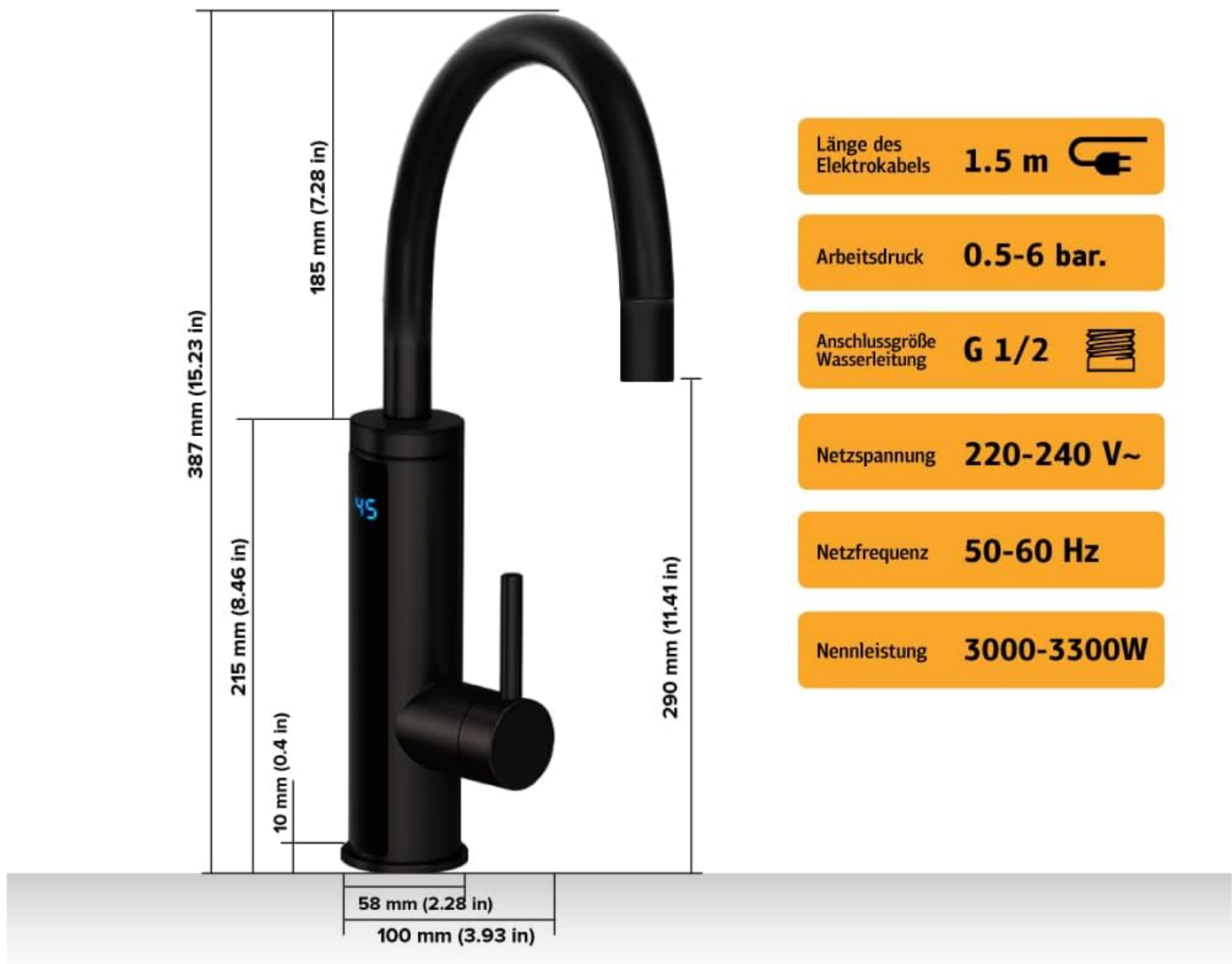
Image 4.2: Detailed diagram providing the physical dimensions of the faucet and key technical specifications such as cable length, operating pressure, water connection size, voltage, frequency, and nominal power.
