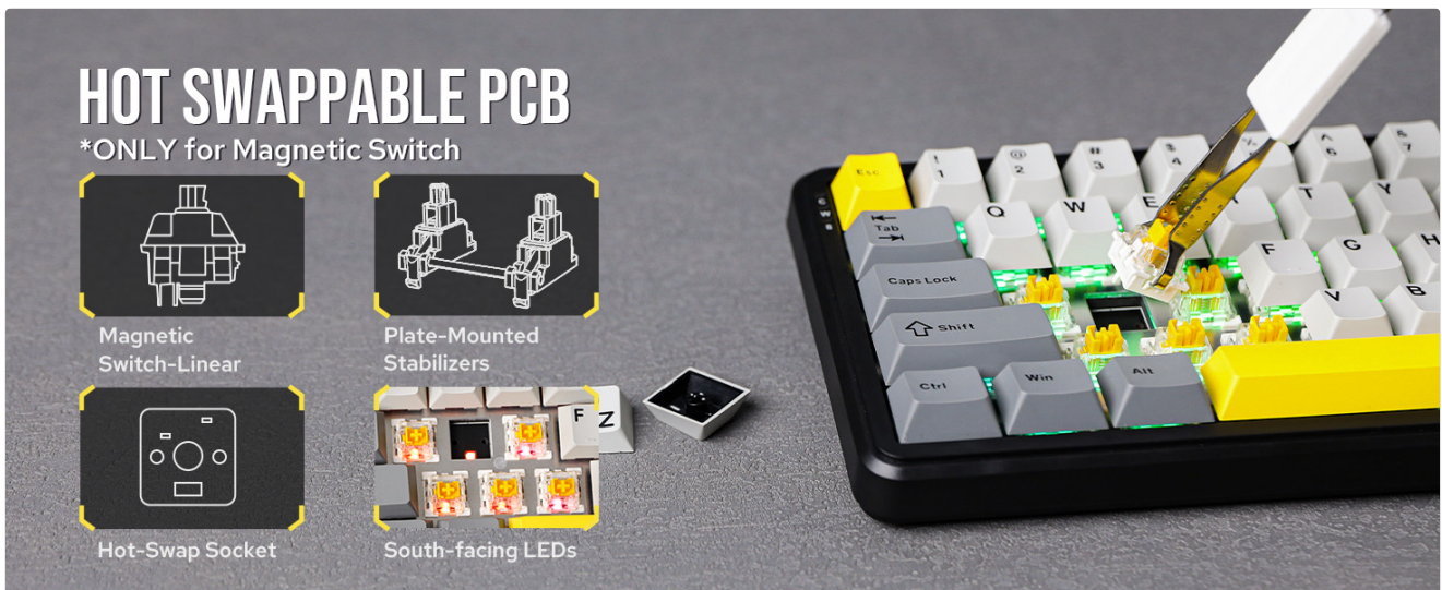
Image 5.1: Illustration of the hot-swappable PCB, magnetic switches, and south-facing LEDs, demonstrating how switches can be replaced.
