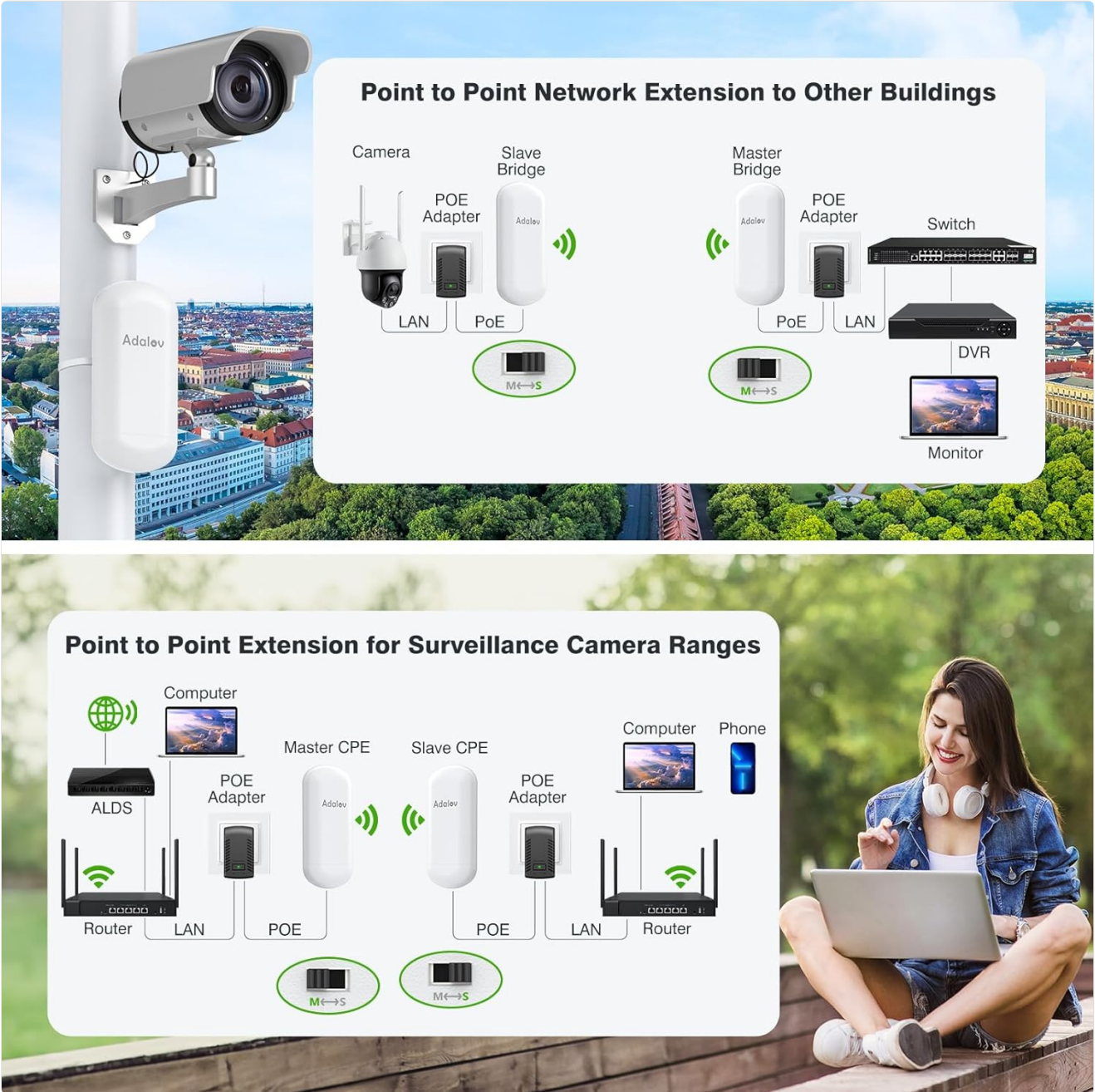
Figure 7: Diagram illustrating a point-to-point network extension setup, connecting a main router to a master bridge, and a slave bridge to a remote network device like a switch or DVR.
