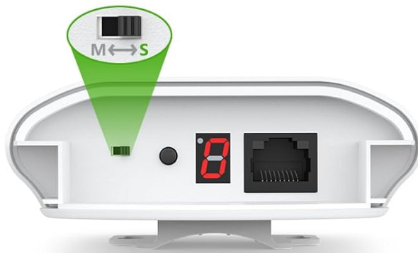
Figure 6: Instructions for single-key operation and auto-pairing: Set Master CPE to A, Slave CPE to B, set the same number/letter on both, and wait for pairing.
